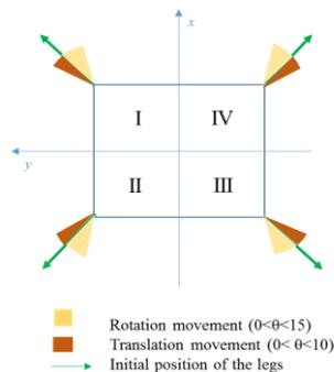
Figure 2. Robot's movement schematic
