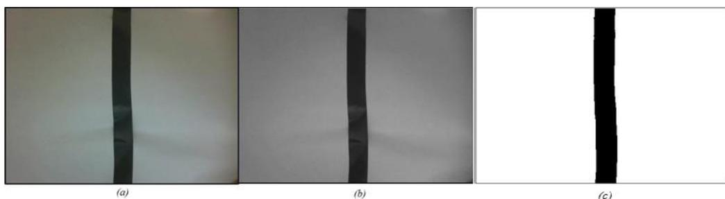
Figure 3. (a) original image; (b) image in gray levels; (c) binary image after applying Otsu Method
