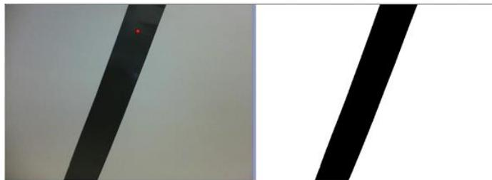
Figure 5: Location of the line center (in red) and binary image using the experimental thresholding method (right)
