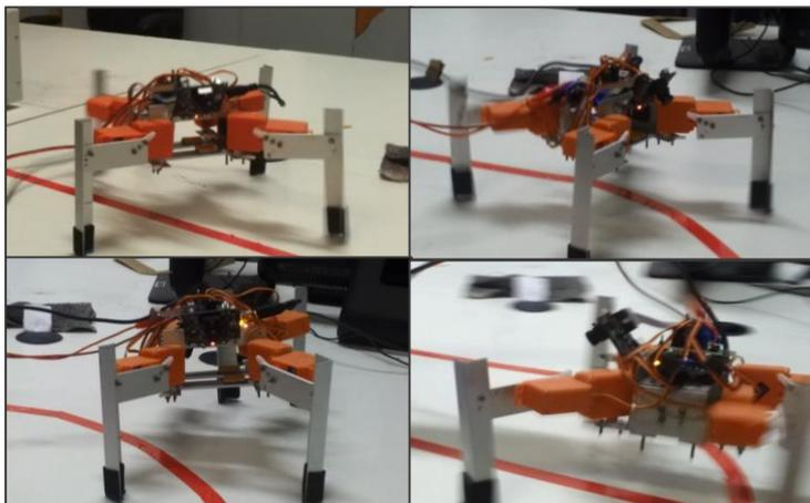
Figure 6: The four-legged line follower robot paired using Pixy camera to follow a delimited path
