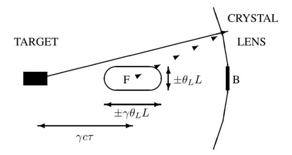
**Fig. 2** Schematic of a target and the focal spot dimensions. The "blind spot" is shown (B).
