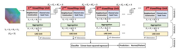
Fig. 1. Illustration of the proposed multi-channel VoxelHop framework, comprising three modules. Our framework utilizes the cascaded multi-stage for local-to-global expansion, akin to the process of CNNs, which has a larger reception field in the deeper layers.
