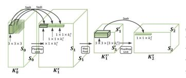
Fig. 4. Illustration of the neighborhood union construction in 3D space and Saab Transform for one channel of 3D data. The same operation is applied to all channels in parallel.
