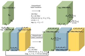
Fig. 3. Illustration of the conventional Saab transform (top) and channel-wise Saab transform for the multi-channel 3D data (bottom).
