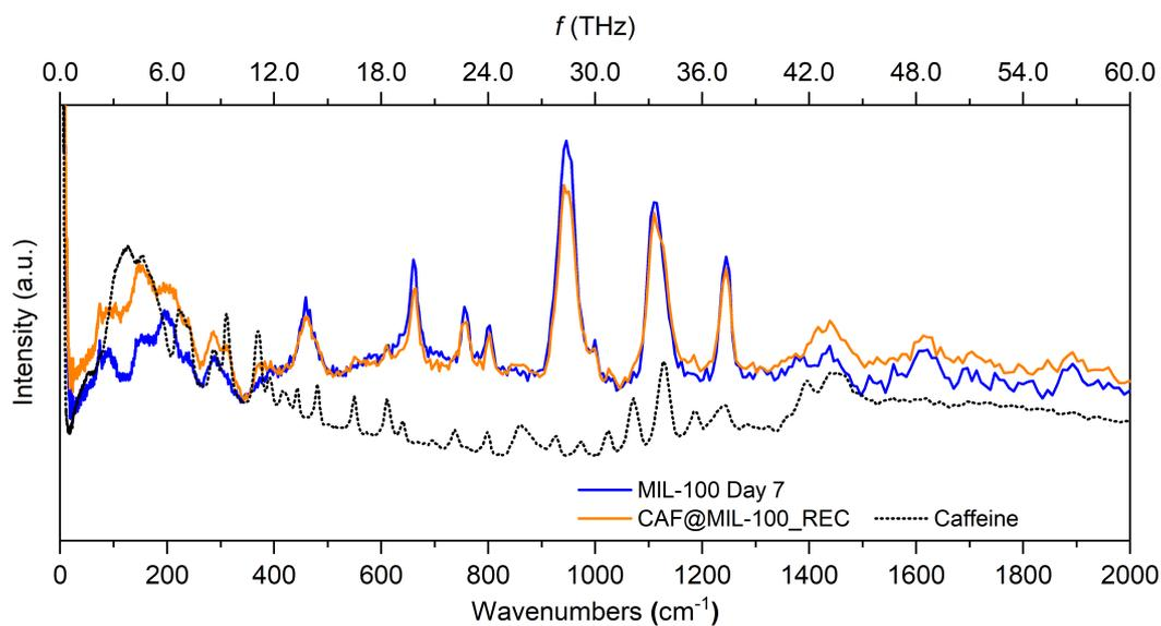
**Figure S18.** INS spectra of CAF@MIL-100 yielded by the reconstruction and *in situ* encapsulation techniques. Spectrum of caffeine presented in black was scaled down by a factor of 0.2 to facilitate the comparison with the guest@MIL-100 systems.
