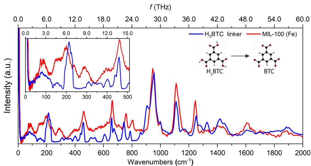
**Figure S11.** INS spectra of pristine MIL-100 (Fe) sample (red) and organic linker H<sub>3</sub>BTC (blue). Good agreement is observed between framework modes and organic linker modes, helping us to pinpoint in the MOF spectrum the vibrational modes related to the organic linker. Note that the H<sub>3</sub>BTC spectrum was scaled down by a factor of 0.3 to facilitate comparison with the MOF spectrum. Colour code: O in red, C in black, and H in grey.
