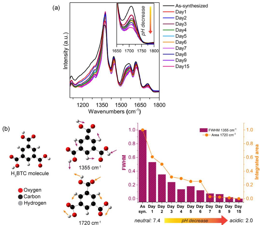
**Figure S2.** (a) Sharpening of the carboxylate vibrational band at  $\sim 1355\text{ cm}^{-1}$  and the decrease in intensity of the C=O stretching of H<sub>3</sub>BTC at  $\sim 1720\text{ cm}^{-1}$ , expressed numerically by (b) FWHM values and integrated area, respectively. Colour code: O in red, C in black, and H in grey.
