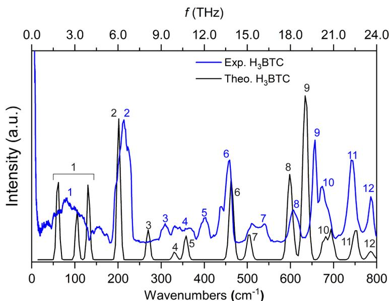
**Figure S10.** Comparison between experimental (blue) and theoretical (black) DFT spectra of H<sub>3</sub>BTC. Numbers were used to facilitate the identification of the vibrational modes. Good agreement between both spectra is observed in the low energy region.
