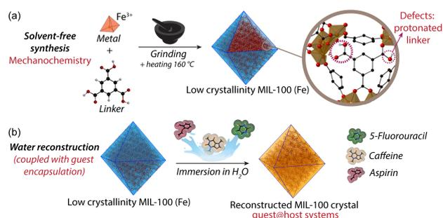
**Figure 1.** Schematic representation of the reconstruction method. (a) Mechanochemical approach applied to the synthesis of low crystallinity MIL-100 (Fe). (b) Reconstruction process to enhance material crystallinity and for the entrapment of different drug molecules within the MOF pores.
