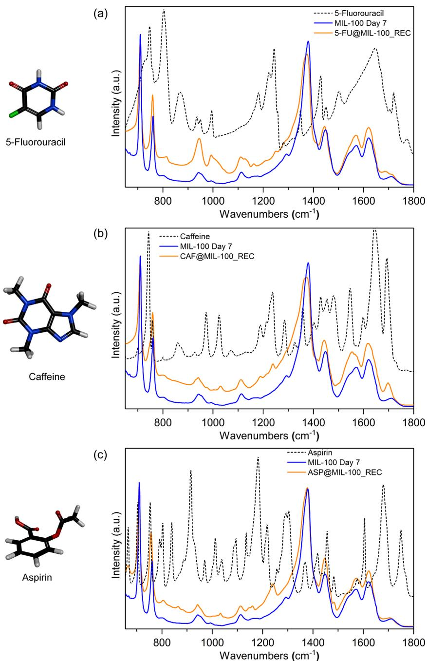
**Figure S20.** ATR-FTIR spectra of guest@host systems displaying (a) 5-FU@MIL-100\_REC, (b) CAF@MIL-100\_REC, and (c) ASP@MIL-100\_REC. For comparison, the spectrum of MIL-100 (Fe) after 7 days of immersion time was also presented. Colour code: O in red, C in black, H in grey, N in navy blue, F in green.
