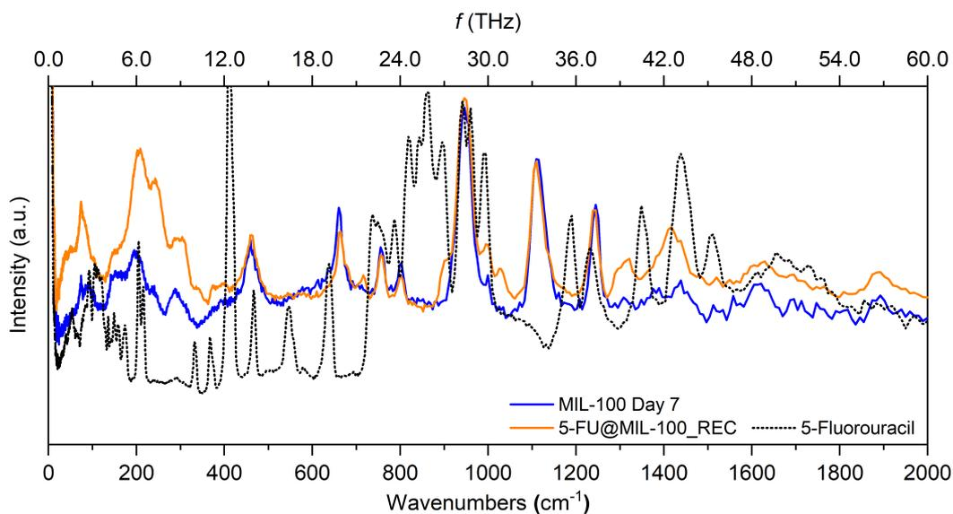
**Figure S17.** INS spectra of 5-FU@MIL-100 yielded by the reconstruction and *in situ* encapsulation techniques. Spectrum of 5-FU presented in black was scaled down by a factor of 0.4 to facilitate the comparison with the guest@MIL-100 systems.
