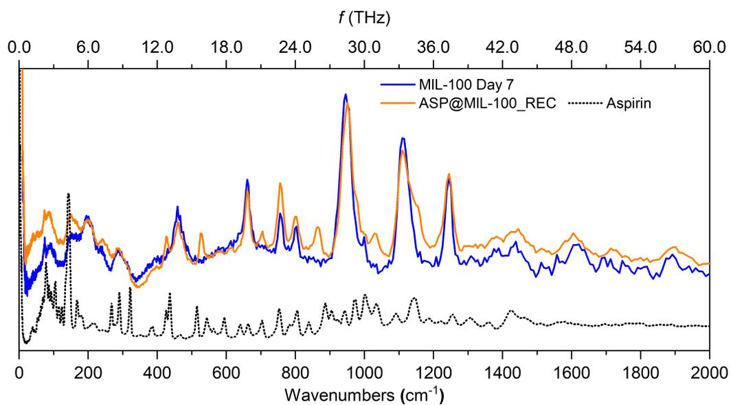
**Figure S19.** INS spectra of ASP@MIL-100 yielded by the reconstruction and *in situ* encapsulation techniques. Spectrum of aspirin presented in black was scaled down by a factor of 0.1 to facilitate the comparison with the guest@MIL-100 systems.
