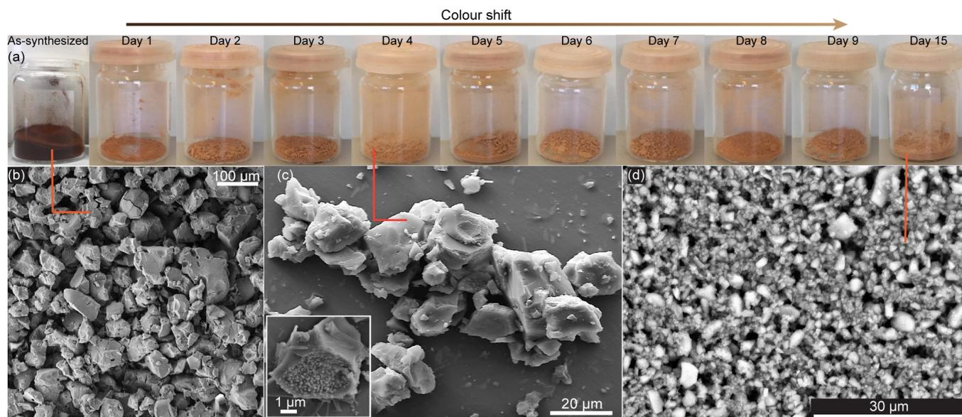
**Figure S4.** SEM images of MIL-100 (Fe) samples. (a) Photographic representation of MIL-100 (Fe) samples collected at different immersion time intervals. The change in the sample color can be associated to changes in the aggregation of particles as observed in (b), (c) and (d), respectively.
