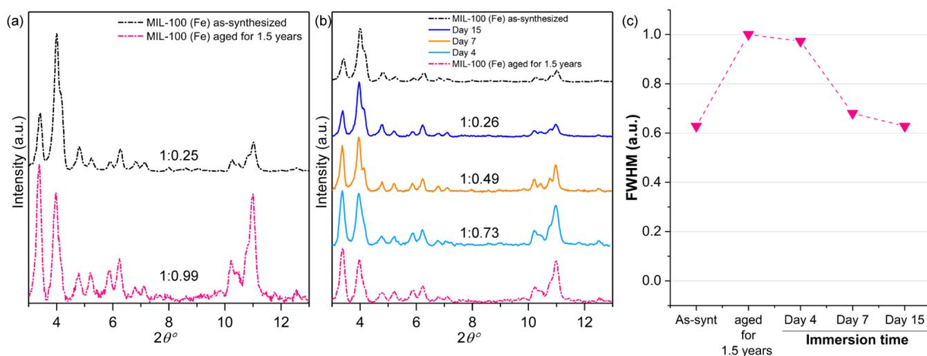
**Figure S6.** PXRD patterns of aged samples used in the reconstruction process. (a) PXRD pattern of fresh MIL-100 (Fe) (black trace) and the aged sample (pink trace). (b) PXRD patterns showing the recovery of crystallinity of the aged sample after immersion in DI water. (c) FWHM of the (022) plane.
