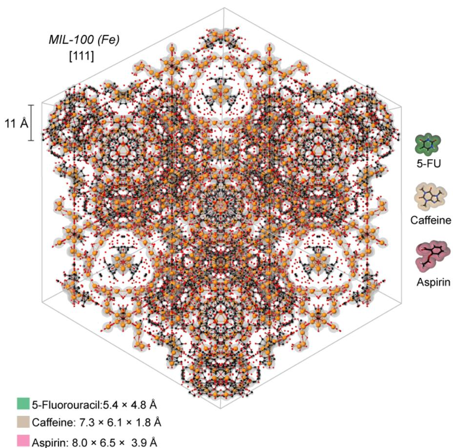
**Figure S24.** Schematic representation of host and guest molecular sizes. The comparison showcases how the mesocages of MIL-100 (Fe) can accommodate multiple of the chosen drug molecules within the MOF pores.
