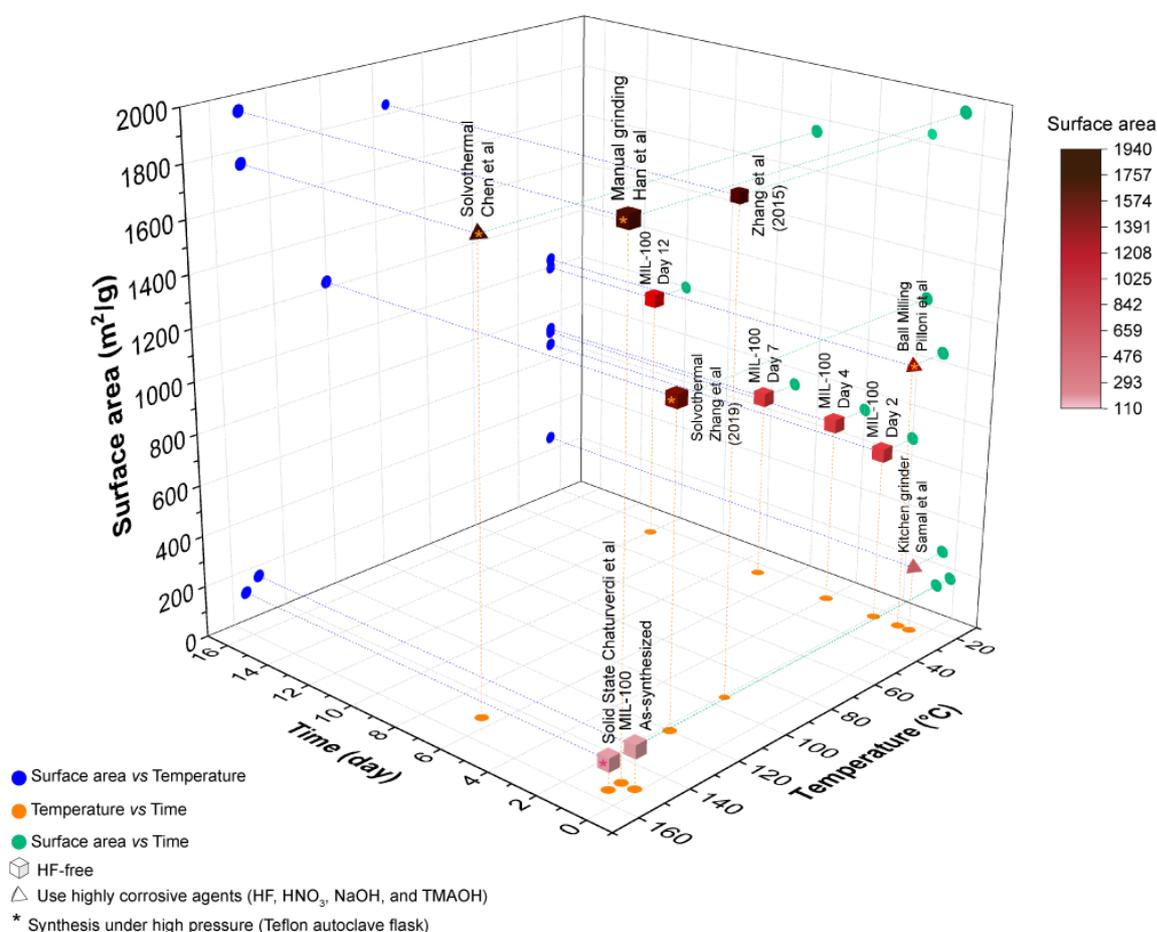
**Figure S3.** Comparison of BET surface area, synthesis temperature and total synthesis time of MIL-100 (Fe) samples prepared in this work *via* the reconstruction technique and the reported BET surface area of MIL-100 (Fe) fabricated *via* various synthetic methods.
