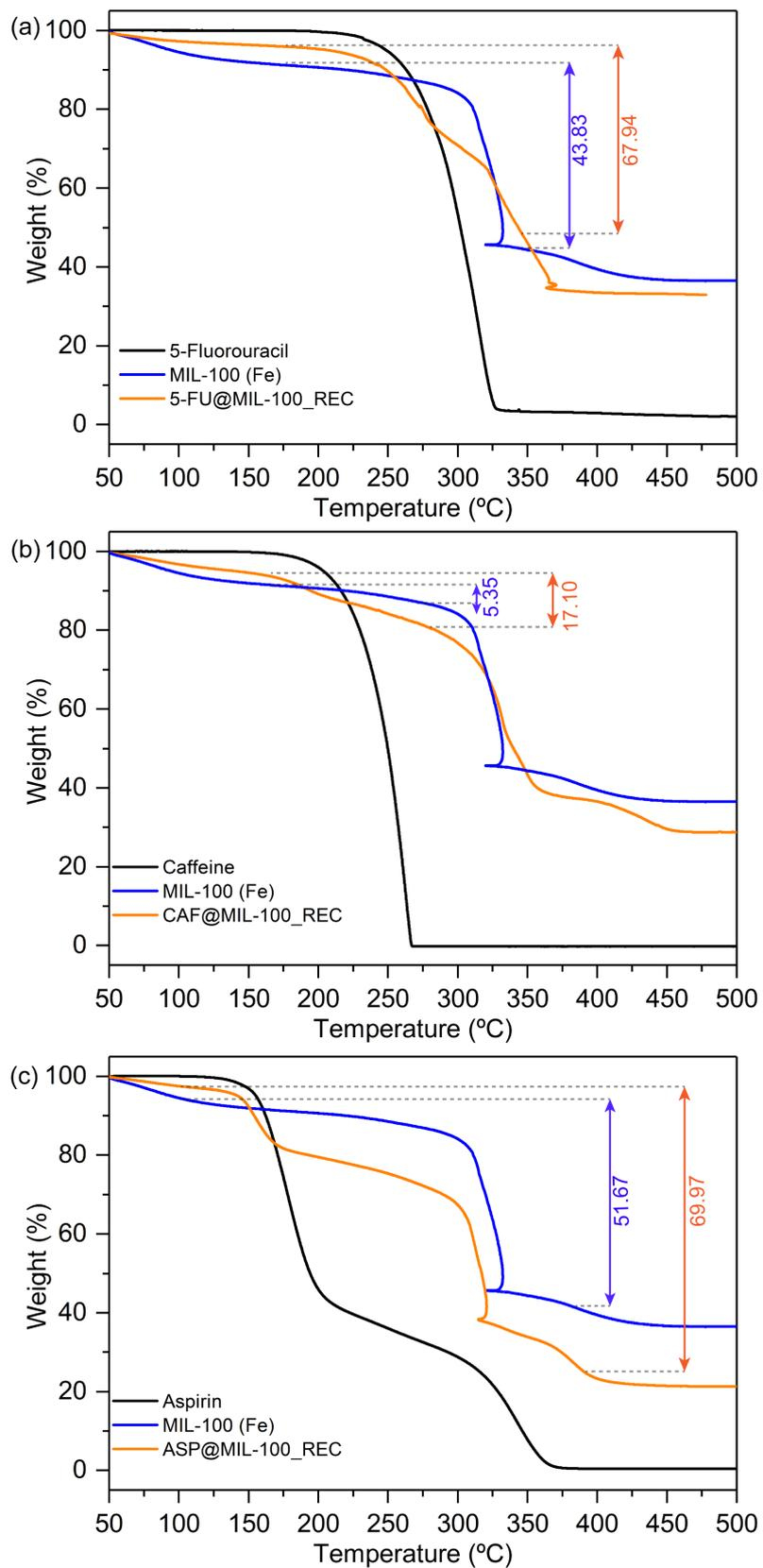
**Figure S22.** TGA of drug@MIL-100 systems showing the material decomposition behaviour as a function of temperature. (a) 5-FU@MIL-100\_REC, (b) CAF@MIL-100\_REC, and (c) ASP@MIL-100\_REC.
