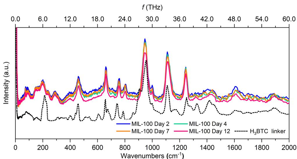
**Figure S16.** INS spectra of MIL-100 (Fe) samples collected after different immersion times. In black is the spectrum of H<sub>3</sub>BTC linker which was scaled down by a factor of 0.2 to facilitate the comparison with MOF spectra.
