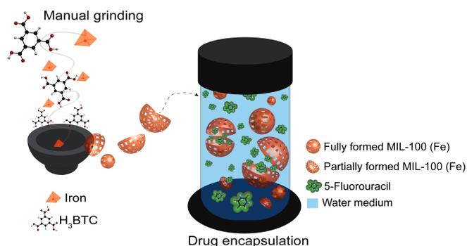
**Figure 6.** Schematic representation of the guest encapsulation mechanism during the reconstruction process immersed in water. The formation of the MOF cages around the drug molecules allows the achievement of high guest loadings.
