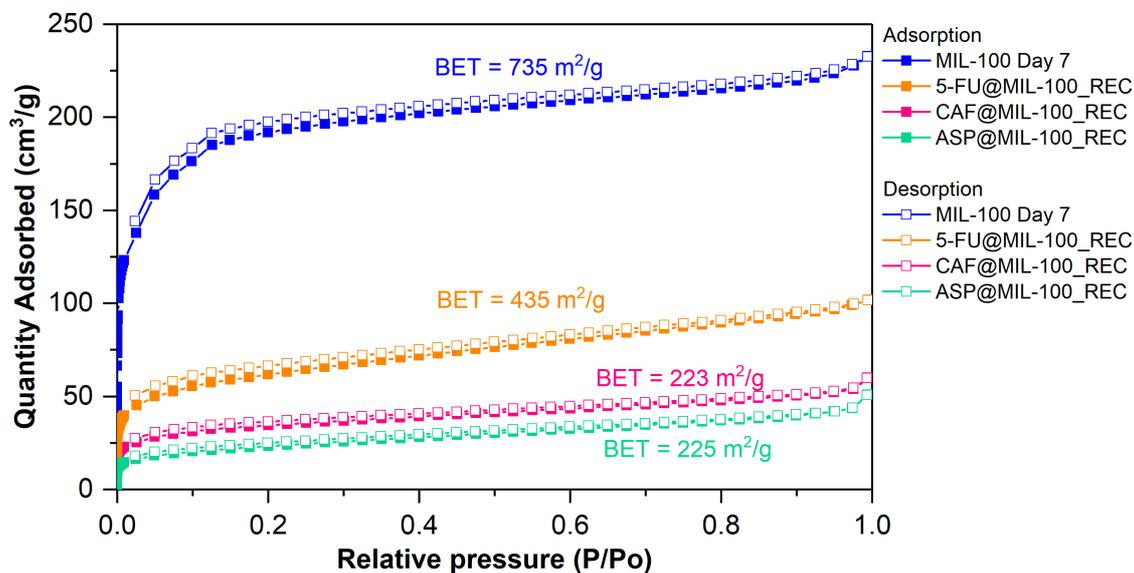
Figure S21. Nitrogen adsorption and desorption isotherms of 5-FU@MIL-100\_REC, CAF@MIL-100\_REC, and ASP@MIL-100\_REC systems.
