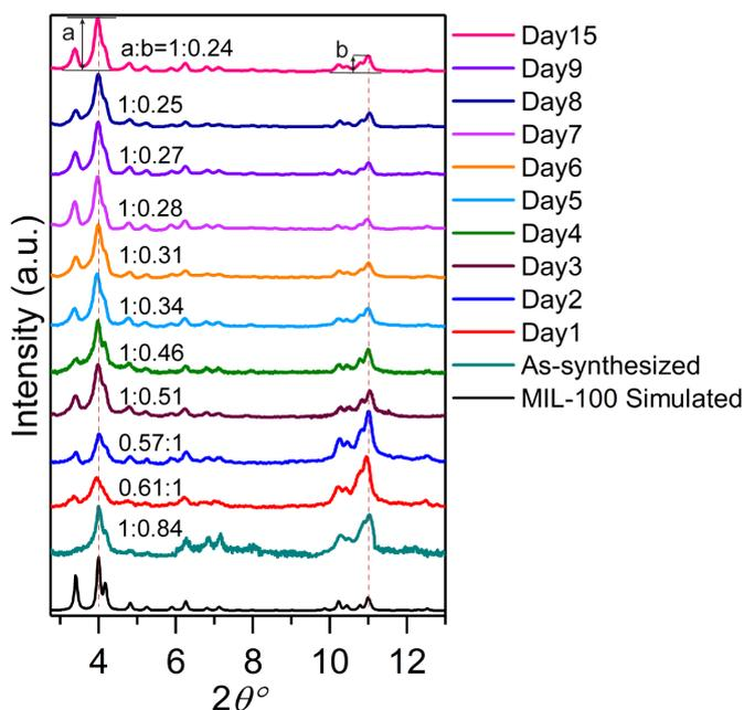
**Figure S1.** Normalized PXRD patterns of MIL-100 (Fe) after different immersion times. Each pattern presents the ratios of the changing relative intensity of the a:b = (022):(357) planes, demonstrating the progressive increase in the relative intensity of the (022) plane.
