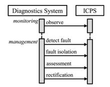
**Fig. 2.** Sequence diagram of diagnostic activities for a generalized ICPS.
