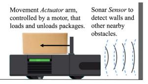
Fig. 1. Sensors and actuators for a warehouse robotic package handler.
