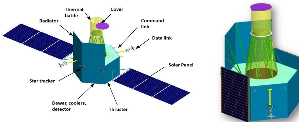
Figure 1. Integrated design of the HUBS spacecraft and payload: (left) with solar panels extended; (right) with solar panels folded. The perspective view of the payload shows the focusing optics assembly, as well as the associated supporting structures, inside the thermal baffle. The dewar is hidden from view.
