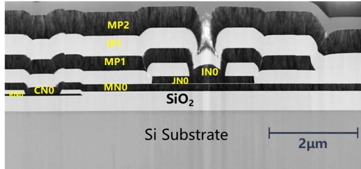
Figure 3. Cross-section of a device fabricated by SIMIT standard fabrication process, courtesy of L.-L. Ying et al.<sup>21</sup>
