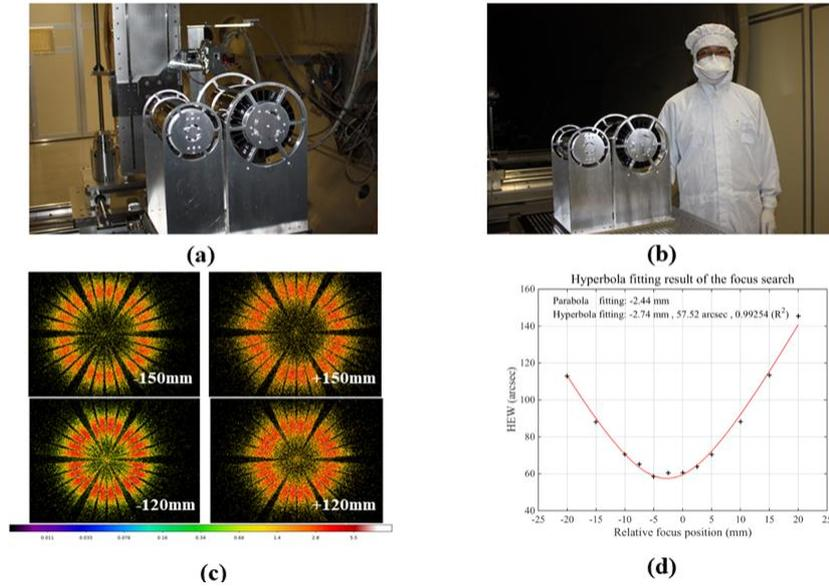
Figure 7. Prototype X-ray telescopes: (top) the photos of 3-layer and 21-layer fully-assembled systems, (bottom) the results of measurements at the PANTER X-ray test facility in Germany.
