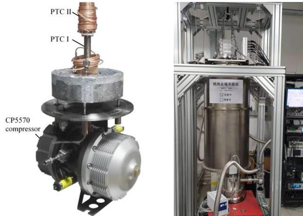
Figure 5. Photos of actual systems: (left) a prototype HFPTC developed at TIPC; (right) a two-stage ADR prototype (hidden inside the dewar) built and tested at Tsinghua University.
