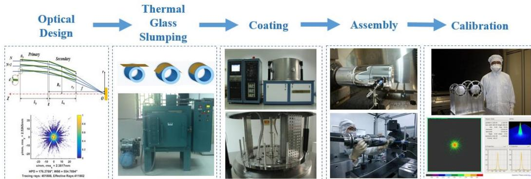
Figure 6. Development of X-ray optics at Tongji University.
