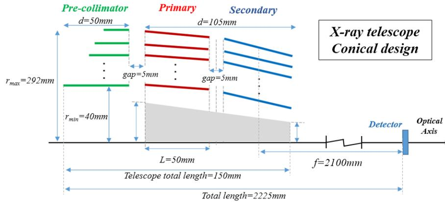
Figure 6. Preliminary design of the HUBS telescope.
