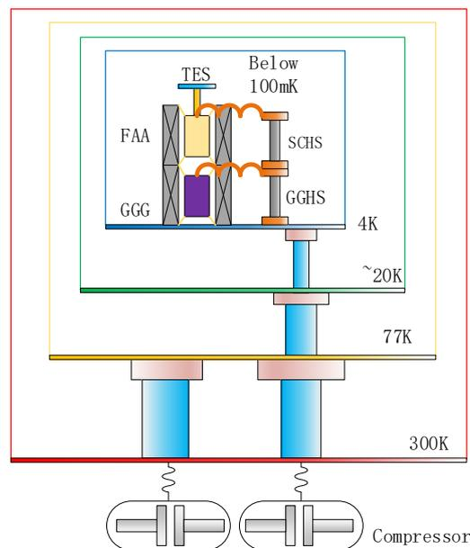
Figure 4. Schematic diagram of the HUBS cooling system. A series of radiation shields are employed at intermediate temperature stages to cut down radiation load from warmer stages.
