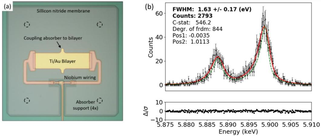
Figure 2. (a) Optical micrograph of a typical SRON TES, labeled with the main components. (b) Energy spectrum of the Mn-K $\alpha$  line complex. The measured spectrum is shown in black, with the solid red line the best-fit model. The green dotted line is the natural line shape. Note that the TES was AC-biased for the measurement.
