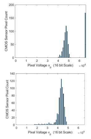
Fig. 5. Histogram plots showing the number of CMOS sensor pixels having specific 16-bit scale individual pixel range  $v_p$  signal outputs. Top plot: 14 dB DR target patch with 169 saturated pixels. Bottom plot: 28 dB target patch with no saturated pixels.
