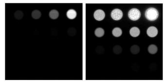
Fig. 8. 78 dB test target images captured for the proposed minimal images multi-exposure method for HDR image recovery. Exposure times are: Left image: 59 µs and Right Image: 5.9 ms.
