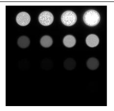
Fig. 4. Single shot image of the 90 dB calibration target used for CRF generation.
