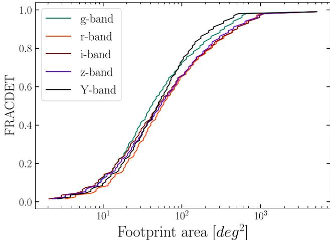
**Figure 7.** Cumulative footprint area as a function of the fractional pixel coverage (FRACDET) on a logarithmic scale. In each band separately, if we select pixels with FRACDET  $> 0.8$  we eliminate  $\sim 130 \text{ deg}^2$  of the survey area.
