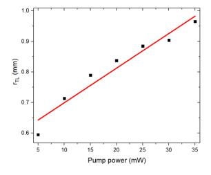
*Figure 6: Dependence of the thermal lens size on the pump power.*
