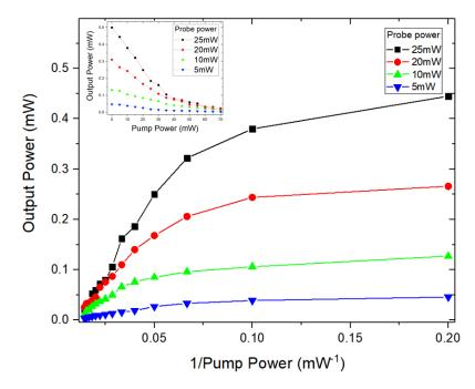
Figure 10:Output characteristics of the "normally on" all optical switch shows output power variation vs 1/(input pump power), inset- output power vs input pump power
