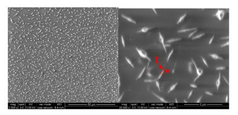
Figure 2: SEM micrograph of thin films of MoS2 nanoflakes dispersion on glass slide. (right)zoomed view.
