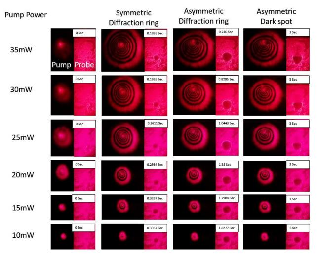
Figure 4: Time evolution of diffraction rings and thermal lens dark spot for different pump power(inset: Elapsed time). See supplementary material for video.
