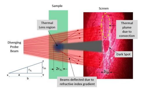
Figure 5: Light rays from the probe beam which encounter thermal lens region get deflected due to refractive index gradient
