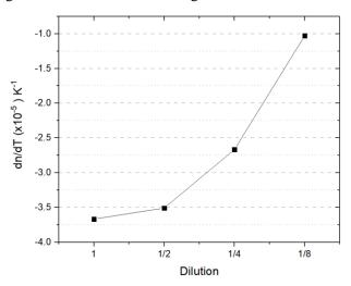
Figure 8: Change in thermal co-efficient of refractive index(dn/dT) for two-fold series dilution of MoS<sub>2</sub> dispersions
