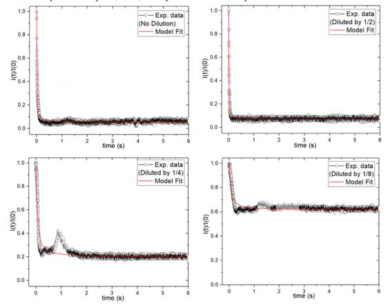
Thermal lens spectroscopic (TLS) analysis of MoS<sub>2</sub> dispersion
