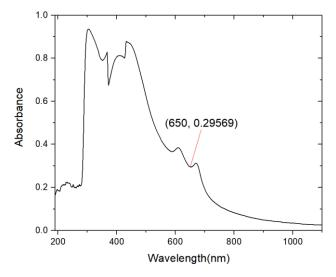
Figure 1:Absorption spectrum of MoS2 nanoflake dispersion.
