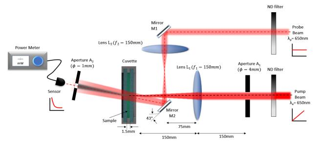
Figure 9: Experimental setup for "normally on" all optical switch (dsitance between  $L_2$  and  $M_2=18cm$ ,  $A_2$  and sample=5cm). Pump beam emerging out of the sample in the cuvette is not shown.
