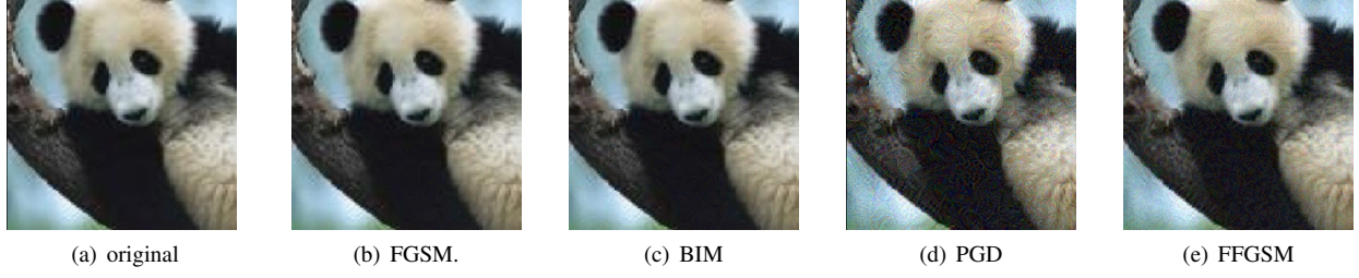
Figure 1: Examples of adversarial images generated by different adversarial attacks for Inception V3 [14]. (a) The original image in ImageNet: classified as “giant panda”; (b) FGSM: classified as “giant panda”; (c) BIM: classified as “standard poodle”; (d) PGD: classified as “toy poodle”; (e) FFGSM: classified as “giant panda”
