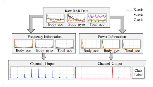
Fig. 5. The feature set corresponding to a sample signal for classification.
