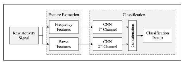
Fig. 1. Proposed CNN-based HAR classification model.
