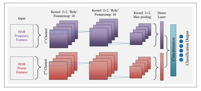
Fig. 6. Proposed two-channel CNN for HAR classification
