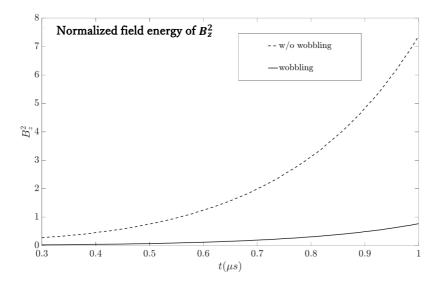
FIG. 10. Histories of normalized field energy of  $B_z^2$  for the sheet electron current plasma systems with (solid line) and without (dotted line) the wobbling or oscillating motion of the sheet electron current along y. The onsets of the filamentation and the magnetic reconnection are delayed and mitigated clearly by the dynamic phase control.
