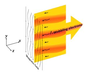
FIG. 6. Schematic diagram for dynamic phase control in electron current sheet sustained plasma system, in which electron filamentation and magnetic reconnection grow. The electron sheet current is oscillated along the sheet, and the perturbation phases introduced by the electron beam smooth and mitigate the perturbation amplitude.
