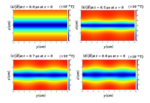
FIG. 3. Distributions of magnetic field strength at x=0 at  $(a)t=0.0\mu s$ ,  $(b)t=0.5\mu s$ ,  $(c)t=0.7\mu s$  and  $(d)t=0.8\mu s$ . Around  $t=0.5\sim0.7\mu s$  the magnetic reconnection becomes distinct.
