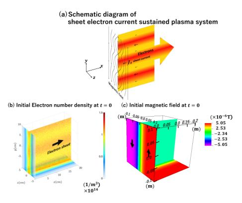
FIG. 1. (a) Schematic diagram of plasma system sustained by sheet electron current. The magnetic reconnection is induced along with the plasma filamentation. The initial conditions of (b) the electron number density  $n_e$  and (c) the magnetic field are also presented. The electron sheet current is located near z=0 and the electrons move in the +x direction. A small electron density perturbation is imposed in  $n_e$  along y.
