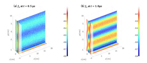
FIG. 5. Distributions of current near the electron current sheet  $J_x$  at (a)  $t=0.5\mu s$  and (b)  $t=1.0\mu s$ . The net current shows the filamentation along with the magnetic reconnection.
