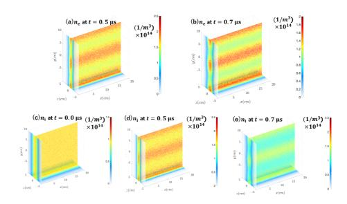
FIG. 2. Spatial distributions of the electron number density  $n_e$  at (a)  $t = 0.5 \mu s$  and (b)  $t = 0.7 \mu s$ , and the proton density  $n_i$  at (c)  $t = 0.0 \mu s$ , (d)  $t = 0.5 \mu s$  and (e)  $t = 0.7 \mu s$ . The electron sheet current is filamented along the z = 0 plane, and the ions also follow the filamentation.
