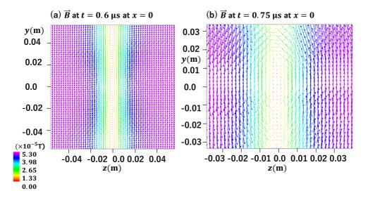
FIG. 4. Distributions of magnetic field vectors at x=0 at (a)  $t=0.6\mu s$  and (b)  $t=0.75\mu s$ . At  $t=\sim 0.5\sim 0.75\mu s$  the magnetic reconnection becomes distinct.
