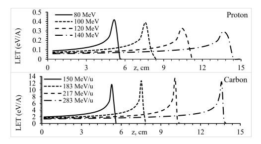
Figure 1. Bragg curves for proton and carbon beams
