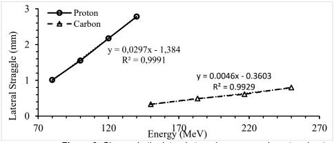
Figure 3. Change in the lateral straggle vs energy in water phantom
