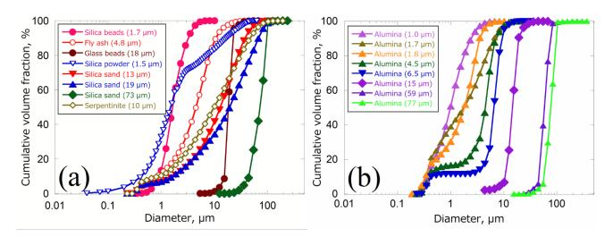
**Figure 1.** Particle size distribution of (a) silica and serpentinite particles and (b) alumina particles. The dust materials used in the mixture samples are shown using blue open triangles and red circles.
