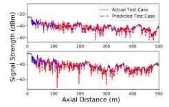
Fig. 9: Predicted versus actual received signal of the same two arbitrarily selected tunnel configurations for the 2.4 GHz case.
