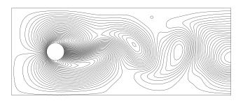
FIGURE 5. Relative streamlines at time  $t = 10, \gamma = 0, \gamma = 10^{-1}, \gamma = 1$  from top.
