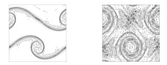
FIGURE 1. Vorticity contours for the double shear layer at time t = 6 and t = 12,  $\gamma = 0$ .
