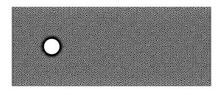
FIGURE 4. Mesh used for vortex shedding computation.
