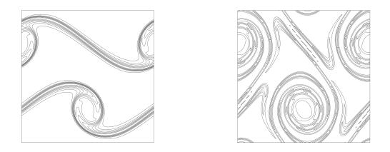
FIGURE 3. Vorticity contours for the double shear layer at time t = 6 and t = 12,  $\gamma = 10^{-1}$ .
