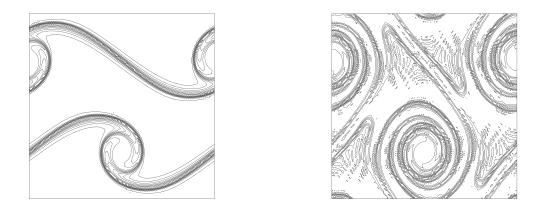
FIGURE 2. Vorticity contours for the double shear layer at time t = 6 and t = 12,  $\gamma = 10^{-2}$ .
