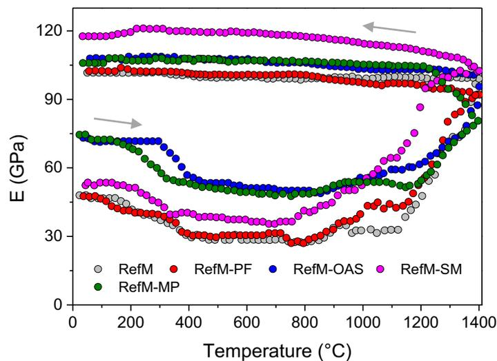
Fig. 9 – Young's modulus evolution as a function of the temperature of the dried samples of the designed castables during their first heating-cooling cycle (30-1400°C). The measurements were carried out with a heating rate of 2°C/min.
