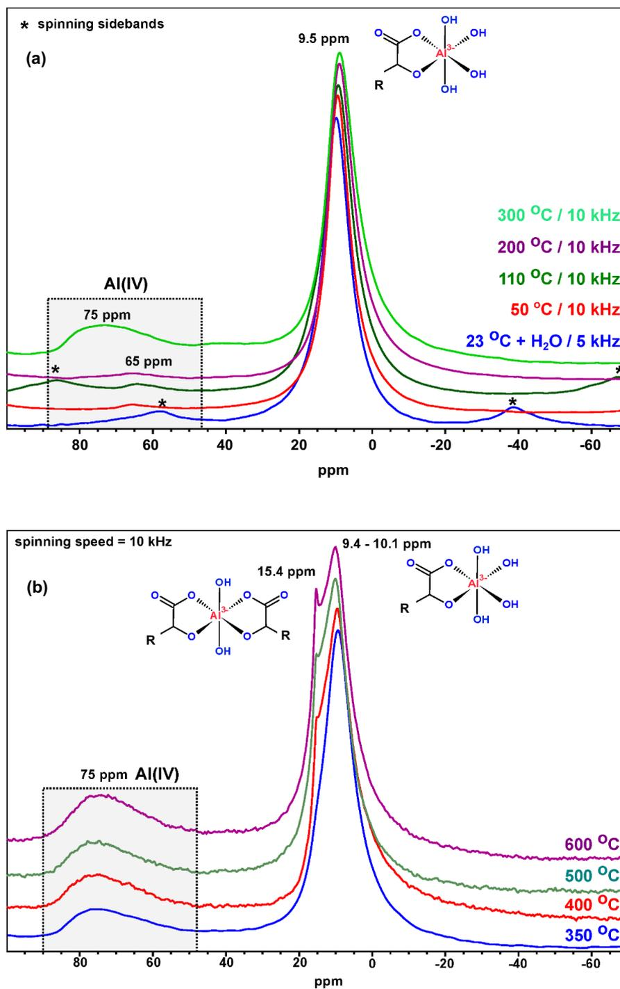
Fig. 2 – <sup>27</sup>Al-ssNMR spectra of MgO-OAS composition after different thermal treatments: (a) curing (30°C or 50°C for 24h), drying (110°C for 24h) or firing at 200°C or 300°C for 2h, and (b) firing in the range of 350°C and 600°C for 2h.
