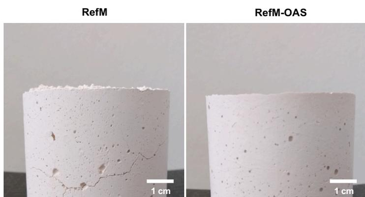
Fig. 8 – Images of the castables' samples obtained after the thermogravimetric tests carried out with a heating rate of 2°C/min and up to 600°C.
