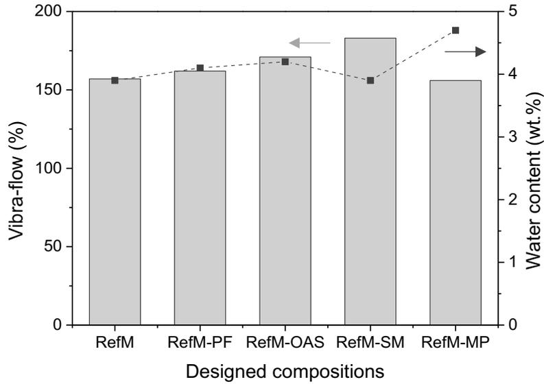
Fig. 4 – Vibratable flow and water demand for the preparation of the designed high-alumina MgO-bonded castables containing different drying agents.
