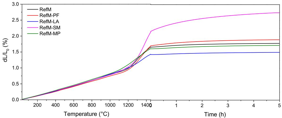
Fig. 10 – Expansion behavior of the designed Al<sub>2</sub>O<sub>3</sub>-MgO castables containing different drying agents. The measurements were carried out with a heating rate of 2°C/min, up to 1450°C for 5h and using an applied load of 0.02 MPa.
