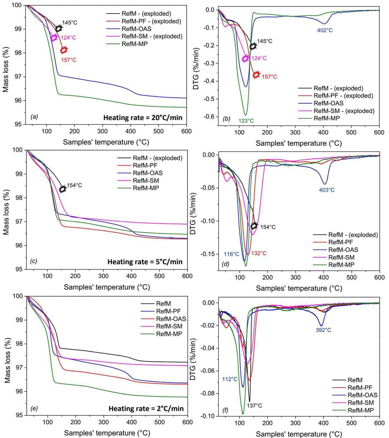
Fig. 7 – (a, c and e) Mass loss (%) and (b, d and f) first derivative of the mass loss curve for the thermal treatments carried out with a heating rate of 20, 5 and 2 °C/min. All samples were cured at 30°C for 1 day before the measurements.
