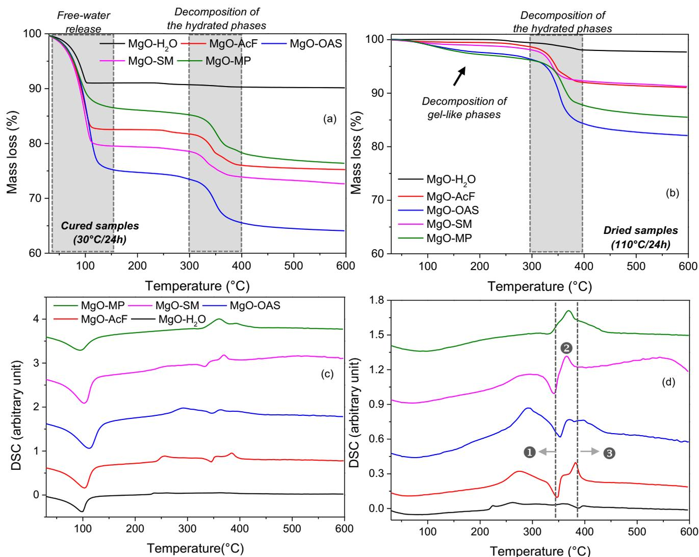
Fig. 1 – Mass loss and DSC profiles of the evaluated MgO-based compositions during their first heating treatment up to 600°C. The samples were kept at (a and c) 30°C/24h or (b and d) 110°C/24h before the measurements. The numbers pointed out in (d) represent: (1) hydrotalcite-like phases, Mg<sub>3</sub>Si<sub>2</sub>O<sub>5</sub>(OH)<sub>4</sub> and/or Mg<sub>3</sub>O(OH)<sub>4</sub> decomposition, (2) desorption of the carboxylic acid and OAS decomposition, and (3) brucite decomposition.
