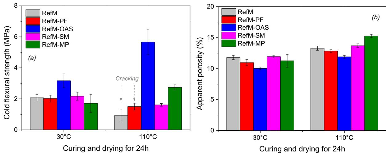
Fig. 6 – (a) Cold flexural strength (3-point bending test) and (b) apparent porosity of the evaluated castables after curing (30°C for 24h) and drying at 110°C for another 24h.
