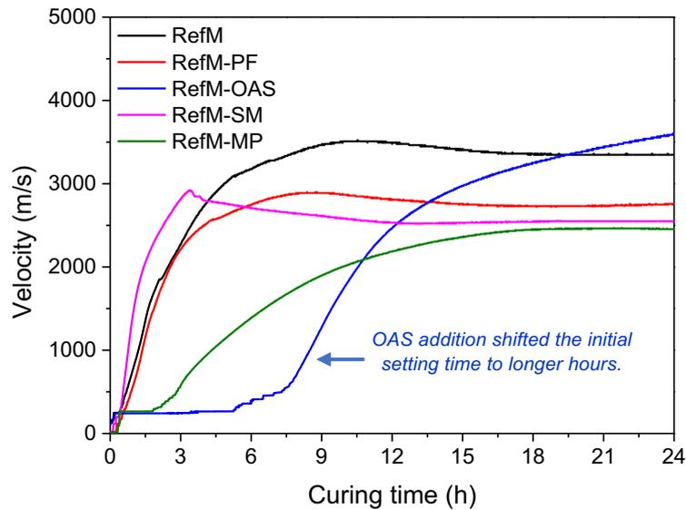
Fig. 5 – Curing behavior of the fresh castable mixes via ultrasonic wave propagation velocity evaluations at 22°C and for 24h.
