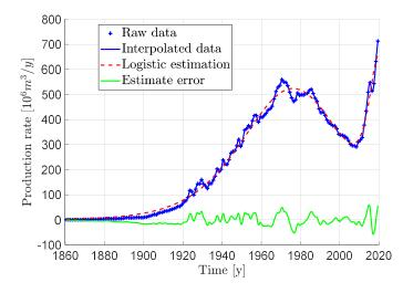
Figure 3. Raw data, estimated logistic rate profile and estimation residuals.
