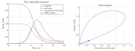
Figure 18. Left: Time profiles of capital stock, resource stock, production and ROI. Right: production-capital phase diagram.
