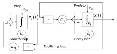
Figure 4. Block-diagram of the LV equation (42).
