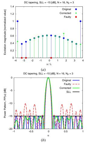
Figure 3. Numerical Assessment (Test Case #1: N = 16,  $N_F = 3 \rightarrow \eta_F \approx 19$  %; DC SLL = -15 [dB]) - Plot of (a) the excitations and of (b) the power patterns of the original, the faulty, and the corrected arrays.
