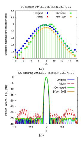
Figure 7. Comparative Assessment (Test Case #3: N = 32,  $N_F = 2 \rightarrow \eta_F = 6.25$  %; DC SLL = -35 [dB]) - Plot of (a) the excitations and of (b) the power patterns of the original, the faulty, and corrected arrays either in [21] or synthesized with the CP method.
