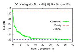
Figure 11. Performance Analysis (DC SLL = -25 [dB]; N = 50;  $\eta_F = 16\%$ ) - Behavior of the side lobe level of the corrected array,  $\widehat{SLL}$ , versus the number of corrections applied,  $\widehat{N}_C$ .
