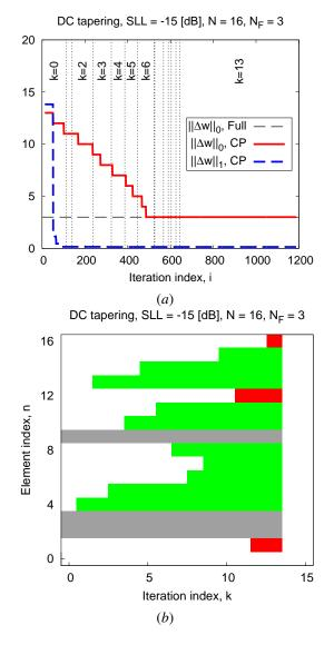
Figure 4. Numerical Assessment (Test Case #1: N = 16,  $N_F = 3 \rightarrow \eta_F \approx 19$  %; DC SLL = -15 [dB]) - Evolution of (a) the  $\ell_1$ -norm and the  $\ell_0$ -norm of the excitation correction vector,  $\Delta \mathbf{w}$ , and of (b) the status ("required/non-required") of the element corrections,  $r_n/s_n$  (n = 1, ..., N), versus the CP iteration index, k.
