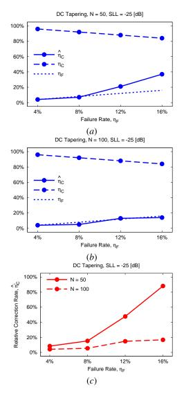
Figure 9. Performance Analysis (DC SLL = -25 [dB]) - Plots of the percentage of failed,  $\eta_F$ , reconfigurable,  $\eta_C$ , and corrected,  $\hat{\eta}_C$ , elements versus the failure rate,  $\eta_F$  in (a) a medium ( $N_1 = 50$ ) and in (b) a large ( $N_2 = 100$ ) array; (c) Behavior of the relative correction rate,  $\hat{\eta}'_C$ , versus  $\eta_F$ .
