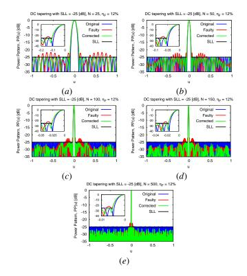
Figure 12. Performance Analysis ( $\eta_F = 12$  %; DC SLL = -25 [dB]) - Plots of the power patterns of the original, the faulty, and the corrected arrays when (a) N = 25, (b) N = 50, (c) N = 100, (d) N = 150, and (e) N = 500.
