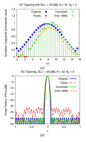
Figure 8. Comparative Assessment (Test Case #4: N = 32,  $N_F = 3 \rightarrow \eta_F \approx 9.4$  %; DC SLL = -35 [dB]; SLL<sub>target</sub> = -35.28 [dB]) - Plot of (a) the excitations and of (b) the power patterns of the original, the faulty, and corrected arrays either in [21] or synthesized with the CP method.
