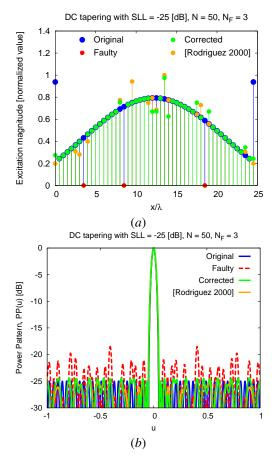
Figure 6. Comparative Assessment (Test Case #2: N = 50,  $N_F = 3 \rightarrow \eta_F = 6$  %; DC SLL = -25 [dB]; SLL<sub>target</sub> = -24.5 [dB]) - Plot of (a) the excitations and of (b) the power patterns of the original, the faulty, and corrected arrays either in [23] or synthesized with the CP method.
