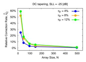
Figure 13. Performance Analysis (DC SLL = -25 [dB]) - Behavior of the relative correction rate,  $\hat{\eta}_C$ , versus N for different values of the failure rate ( $\eta_F \in \{4, 8, 12\}$  %).
