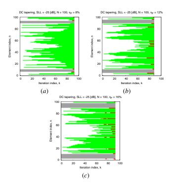
Figure 10. Performance Analysis ( $N_2 = 100$ ; DC SLL = -25 [dB]) -Evolution of the backtracking vectors versus the CP iteration index when (a)  $\eta_F = 8$  %, (b)  $\eta_F = 12$  %, and (c)  $\eta_F = 16$  %.
