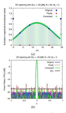
Figure 5. Comparative Assessment (Test Case #2: N = 50,  $N_F = 3 \rightarrow \eta_F = 6$  %; DC SLL = -25 [dB]; SLL<sub>target</sub> = -22.4 [dB]) - Plot of (a) the excitations and of (b) the power patterns of the original, the faulty, and corrected arrays either in [23] or synthesized with the CP method.
