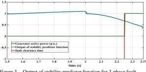
Figure 3. Output of stability predictor function for 3-phase fault
