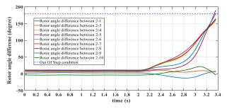
Fig. 5 Rotor angle difference of generators during 2-phase fault
