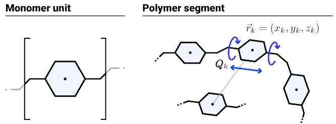
FIG. 1. Polymeric materials are here modelled as a network of  $N$  nodes, each of which represents a monomer. Monomers positions  $\vec{r}_k$  and conformational coordinates  $Q_k$  define the morphology of the medium and the structure of the exciton's Hamiltonian. Exciton transport on such network is mediated by through-bond couplings between conjugated monomers that are part of the same polymer, or by through-space couplings (*gray line*) between pairs of monomers in proximity of each other.
