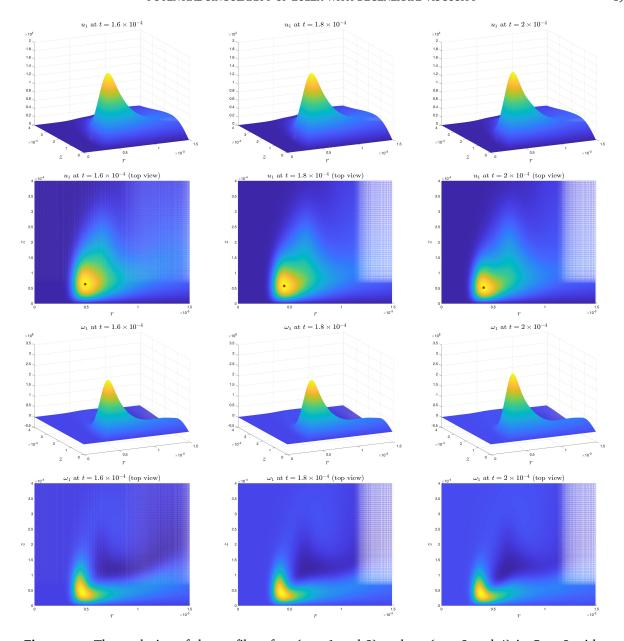
**Figure 5.1:** The evolution of the profiles of  $u_1$  (row 1 and 2) and  $\omega_1$  (row 3 and 4) in Case 2 with  $\nu^r = \nu^z = 10^{-5}$ . Line 1 and 3 are the profiles of  $u_1$ ,  $\omega_1$  at three different times; Line 2 and 4 are the corresponding top-views. The red dot is the location of maximum point of  $u_1$ .
