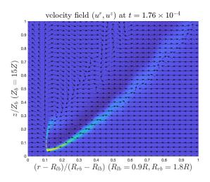
**Figure C.3:** Directions of the velocity  $(u^r, u^z)$  (vectors) and the profile of  $\omega_1$  (background color map) in rescaled coordinates at  $t = 1.76 \times 10^{-4}$ . The velocity field has a strong shearing along the tail of  $\omega_1$ .
