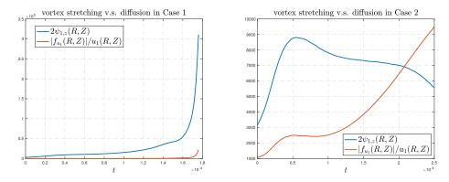
**Figure 5.4:** The relative magnitudes of the vortex stretching  $2\psi_{1,z}$  and the viscosity  $|f_{u_1}|/u_1$  at the point (R(t), Z(t)) in Case 1 (left) and in Case 2 (right).
