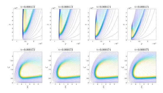
**Figure 7.4:** Comparison of the level sets of  $u_1$  at different time instants. First row: original level sets of  $u_1$  in the domain  $(r, z) \in [0.8 \times 10^{-4}, 2.5 \times 10^{-4}] \times [0, 8 \times 10^{-6}]$ . Second row: rescaled level sets of  $u_1$  as a function of  $(\xi, \zeta)$  in the domain  $(\xi, \zeta) \in [-2, 5] \times [0, 3.5]$ .
