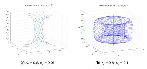
**Figure 3.7:** The streamlines of  $(u^r(t), u^\theta(t), u^z(t))$  at time  $t = 1.7 \times 10^{-4}$  with initial points given by (a)  $(r_0, z_0) = (0.8, 0.01)$  and (b)  $(r_0, z_0) = (0.8, 0.1)$ . The green pole is the symmetry axis r = 0.
