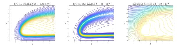
**Figure 7.7:** Level sets of the stretched functions  $\tilde{u}_1$  (left),  $\tilde{\omega}_1$  (middle) and  $\tilde{\phi}_1$  (right) at  $t = 1.76 \times 10^{-4}$ .
