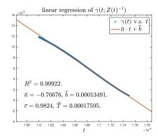
**Figure 7.3:** The linear regression of  $\gamma(t; R(t)^{-1})$  (left) and  $\gamma(t; Z(t)^{-1})$  (right) on the time interval  $[t_1, t_2] = [1.65 \times 10^{-4}, 1.75 \times 10^{-4}]$ . The blue points are the data points obtained from our computation, and the red lines are the linear models. We plot the linear models on a larger interval.
