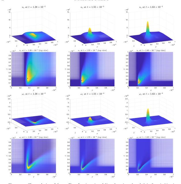
**Figure 3.1:** The evolution of the profiles of  $u_1$  (row 1 and 2) and  $\omega_1$  (row 3 and 4) in Case 1. Line 1 and 3 are the profiles of  $u_1$ ,  $\omega_1$  at three different times; Line 2 and 4 are the corresponding top-views. The red dot is the location of the maximum point of  $u_1$ .
