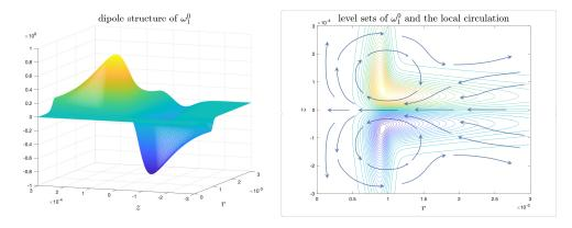
**Figure 3.11:** The dipole structure of the initial data  $\omega_1^0$  and the induced local velocity field.
