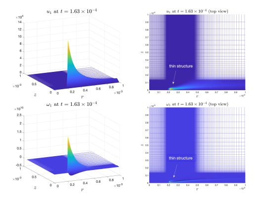
**Figure 3.4:** Profiles and level sets of  $u_1$  (first row) and  $\omega_1$  (second row) at time  $t = 1.63 \times 10^{-4}$  in the square domain  $\{(r, z) : 0 \le r \le 10^{-3}, 0 \le z \le 10^{-3}\}$ .
