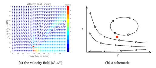
**Figure 3.9:** (a) The velocity field  $(u^r(t), u^z(t))$  near the maximum point (R(t), Z(t)) of  $u_1(t)$  (the red point) at  $t = 1.7 \times 10^{-4}$ . The color corresponds to the magnitude of  $\sqrt{(u^r)^2 + (u^z)^2}$ . The size of the domain has been rescaled. (b) A schematic of the vector field near the point (R(t), Z(t)).
