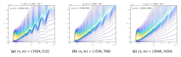
**Figure C.2:** Contours of  $u_1$  at  $1.764 \times 10^{-4}$  with different resolutions. The tail oscillations become weaker as the resolution of the numerical solution increases.
