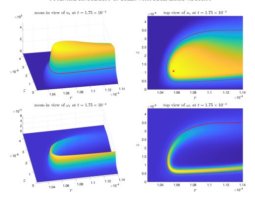
**Figure 3.5:** Zoom-in views of  $u_1$ ,  $\omega_1$  at time  $t = 1.75 \times 10^{-4}$ . First row: profile and tow view of  $u_1$ . Second row: profile and top view of  $\omega_1$ . The red curve (in all figures above) is the level set of  $u_1$  for the value  $0.3||u_1||_{L^{\infty}}$ , and the red point is the maximum point of  $u_1$ .
