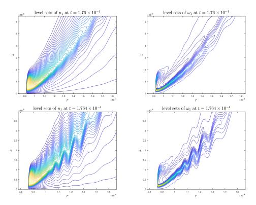
**Figure C.1:** The level sets of  $u_1$ ,  $\omega_1$  in Case 1 at  $t=1.76\times 10^{-4}$  (first row) and  $t=1.764\times 10^{-4}$  (second row). There oscillations begin to appear at  $t=1.76\times 10^{-4}$  and become severer at  $t=1.764\times 10^{-4}$ .
