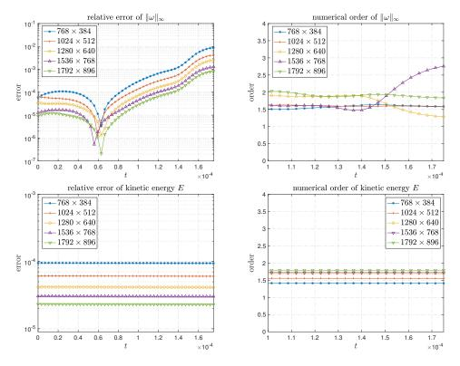
**Figure 4.5:** First row: relative error and numerical order of  $\|\omega(t)\|_{L^{\infty}}$ . Second row: relative error and numerical order of E(t). The last time instant shown in the figure is  $t = 1.76 \times 10^{-4}$ .
