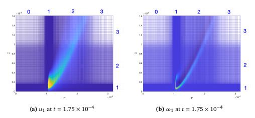
**Figure 4.2:** The adaptive mesh has different densities in different phases. The blue numbers are the labels of the phases.
