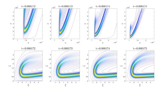
**Figure 7.5:** Comparison of the level sets of  $\omega_1$  at different time instants. First row: original level sets of  $u_1$  in the domain  $(r, z) \in [0.8 \times 10^{-4}, 2.5 \times 10^{-4}] \times [0, 8 \times 10^{-6}]$ . Second row: rescaled level sets of  $\omega_1$  as a function of  $(\xi, \zeta)$  in the domain  $(\xi, \zeta) \in [-2, 5] \times [0, 3.5]$ .
