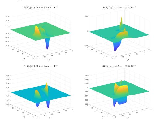
**Figure 4.3:** First row: the mesh effectiveness functions of  $u_1$  at  $t = 1.75 \times 10^{-4}$  with mesh dimension (n, m) = (1024, 512). Second row: the mesh effectiveness functions of  $\omega_1$  in the same setting.
