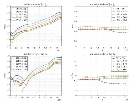
**Figure 4.4:** First row: relative error and numerical order of  $||u_1(t)||_{L^{\infty}}$ . Second row: relative error and numerical order of  $||\omega_1(t)||_{L^{\infty}}$ . The The last time instant shown in the figure is  $t = 1.76 \times 10^{-4}$ .
