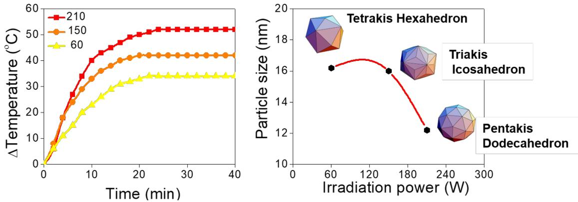
**Fig. 4.** Left panel: Temperature increase as a function of time along the reaction process for samples labeled 60, 150 and 210. The stabilization of the reaction temperature was observed after approximately 20 minutes from the start of the irradiation. Right panel: illustration of the changes in polyhedron shapes adopted by GNPs and the corresponding average particle sizes vs. nominal irradiation power.
