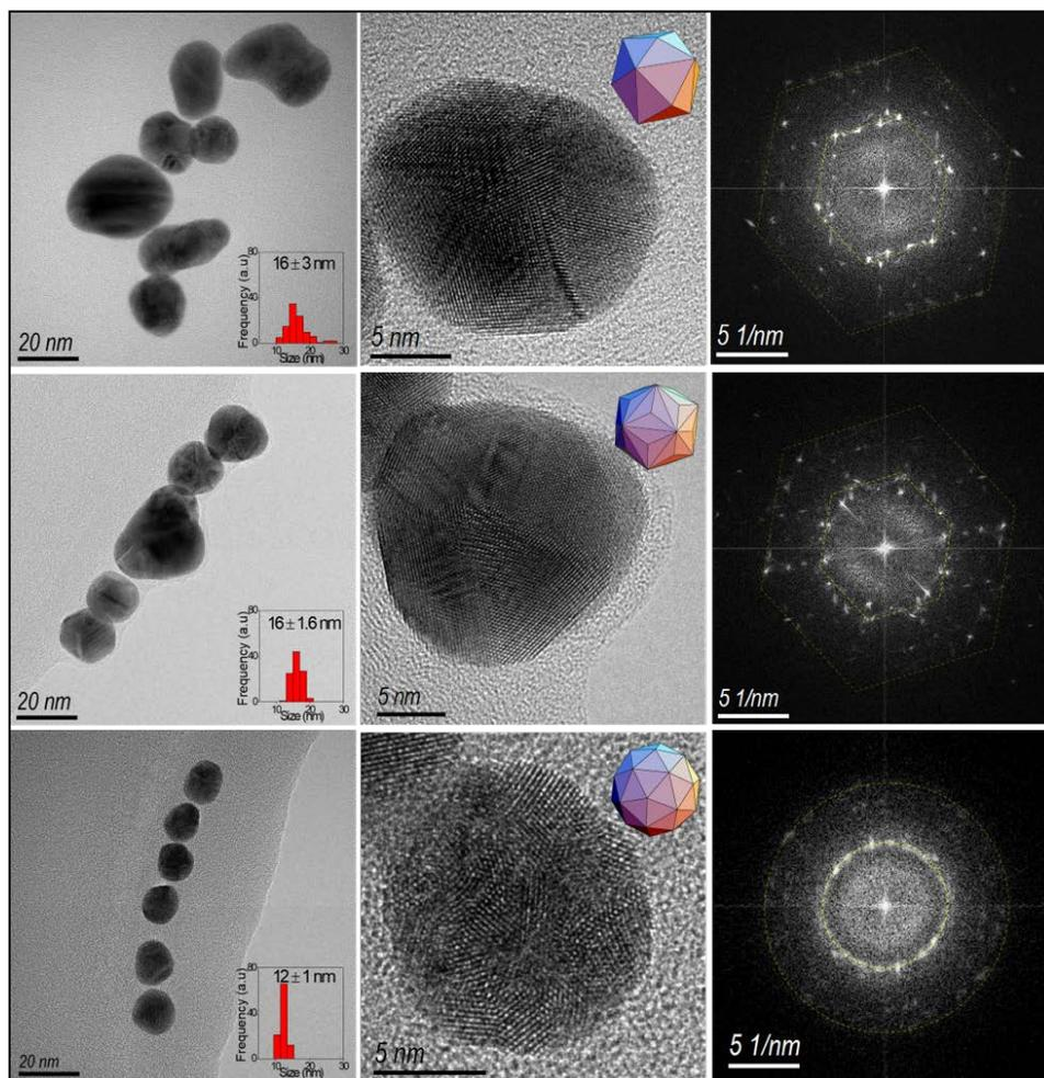
**Fig. 3.** In the first column, the (a), (d), and (g) TEM micrographs of nanoparticles, in the insets, histograms of size distribution are the showed. In the second column (b), (e) and (h) are HRTEM micrographs, insets are polyhedral. The third column (c), (f), and (i) allows us to observe the SAEDs.
