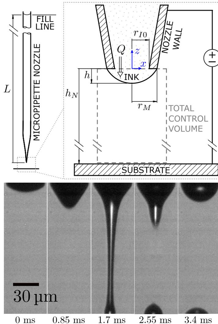
Figure 2.1: (*Top*) Schematic of e-jet printing setup. Dimensions represent signed displacements in the direction of the single-sided arrows with respect to the inertial  $(x, z)$  coordinate system. The volumetric flow rate  $Q$ , labeled via block arrow, is also a signed quantity, but its sign is with respect to the control volume denoted by the dashed box. (*Bottom*) Time lapse photography of an ejection with time stamps from the rising edge of a voltage pulse.
