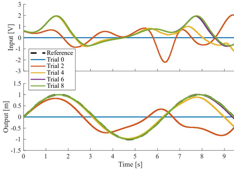
Figure 3.5: Timeseries evolution over multiple trials for a simulation with  $\|e_\theta\|_2 = 0.27$ . This simulation took 8 trials to completely converge.
