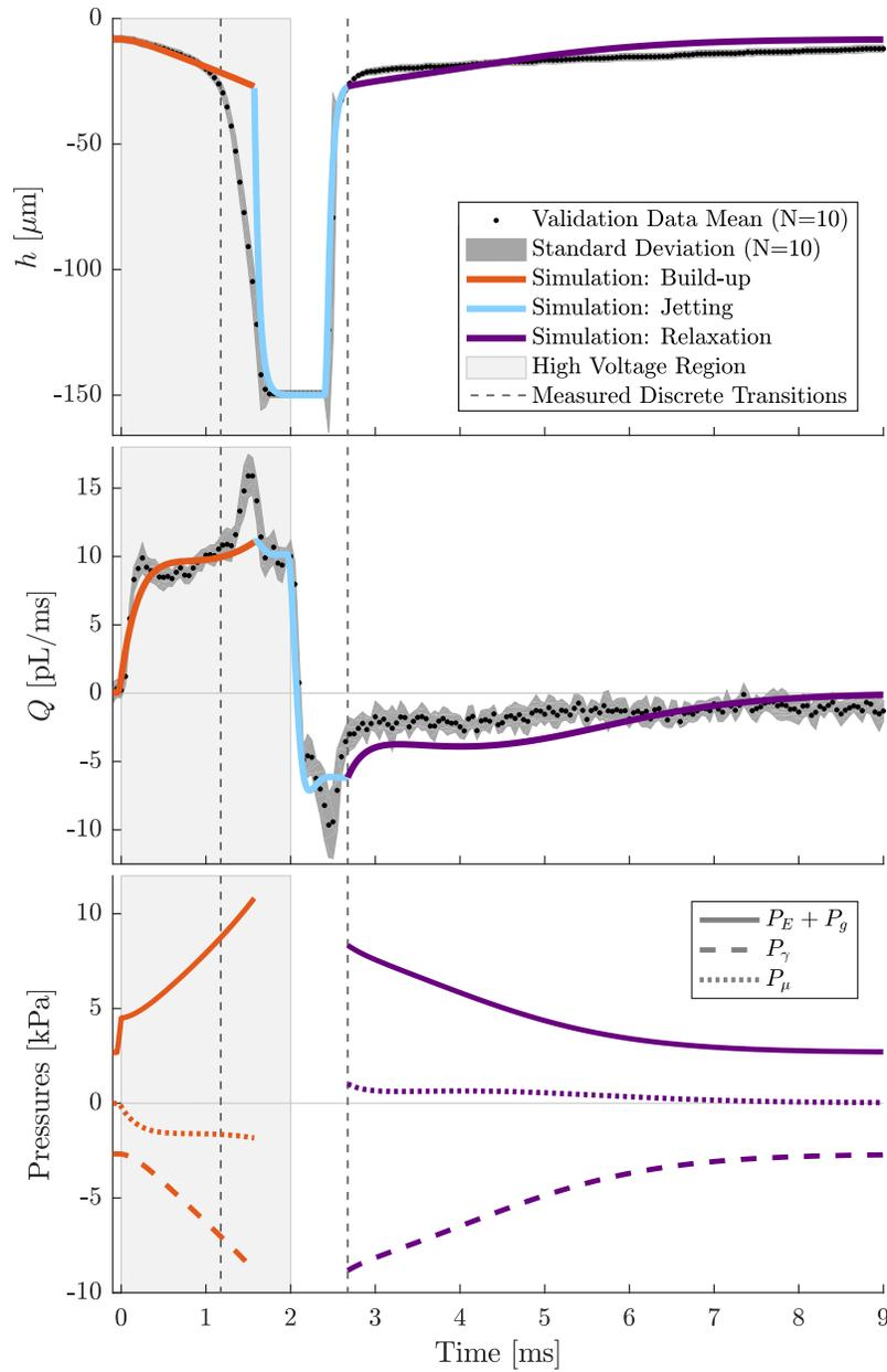
Figure 2.8: Plot of the simulation and measured data for  $h$ ,  $Q$ , and the individual pressure components contributing to  $Q$  for  $T_p = 2$  ms and  $V_h = 1150$  V.  $P_E$  and  $P_g$  are combined because  $P_g$  is constant and they are both always positive, meaning that their sum should be balanced against  $P_\gamma$  with the assistance of  $P_\mu$ .
