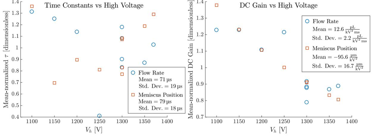
Figure 2.6: Time constants ( $\tau$ ) and DC Gains ( $G$ ) of  $Q$  and  $h$  jetting models versus  $V_h$ . For comparability between  $Q$  and  $h$ ,  $\tau$  and  $G$  are normalized by their mean value. No correlation is apparent between  $\tau$  and  $V_h$ . However, DC Gain and  $V_h$  are clearly correlated.
