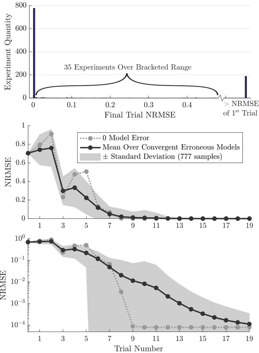
Figure 3.4: *Above*: Histogram of final-trial NRMSE for all experiments. All but the highest error bin are defined by a 0.005 range of NRMSE. *Middle*: Average trajectory of NRMSE vs. Trial number for all completely convergent simulations. *Bottom*: Same on a logarithmic scale, for perspective.
