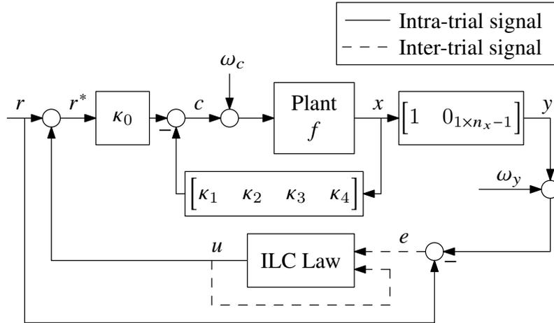
Figure 4.3: System Block Diagram. The control law outputting  $u$  is synthesized from the control models defined by the behatted parameters of Table 4.1 and by  $\omega_c(k) = \omega_y(k) = 0$ . The plant and controller gain blocks are defined with the truth model parameters generated according to Section 4.4.3. Inter-trial signals from trial  $\ell$  are stored and used to compute the input for trial  $\ell + 1$ .
