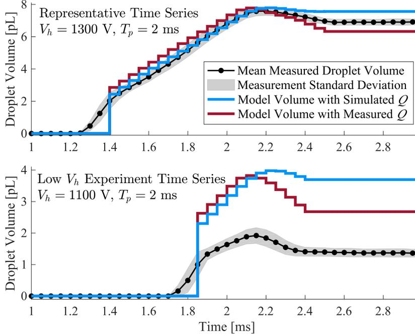
Figure 2.16: Time series plots of droplet volume  $\mathcal{V}_d$  for a representative experiment and the experiment of lowest high voltage  $V_h$ . Plotted measured data is the mean of the validation data ( $N = 10$  samples for each time series) with an envelope of plus or minus the standard deviation. The data suggests that the reset is the main source of error in low  $V_h$  experiments.
