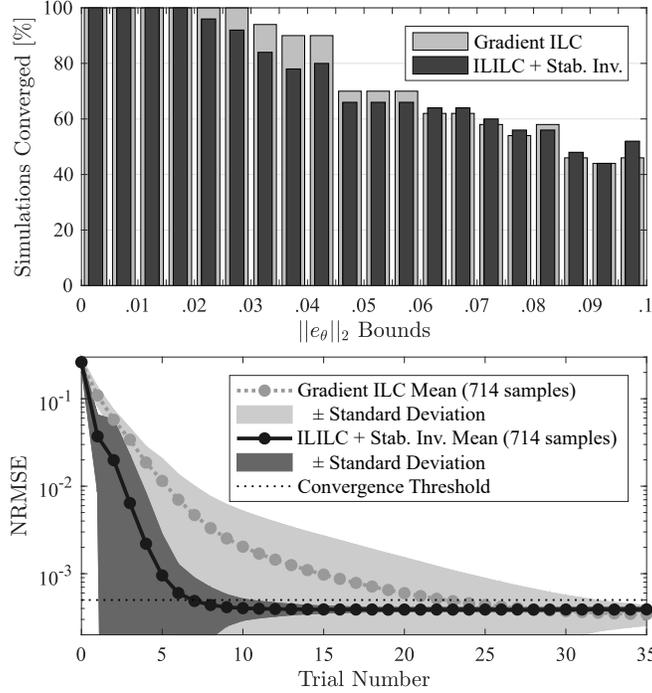
Figure 4.5: *Top*: Histogram giving the percentage of simulations converged in each bin of the model error metric  $\|e_\theta\|_2$ . *Bottom*: Mean value of NRMSE for each ILC trial over all simulations that are convergent for both gradient ILC and ILILC with stable inversion. This illustrates that for comparable robustness to model error, ILILC converges substantially faster than gradient ILC.
