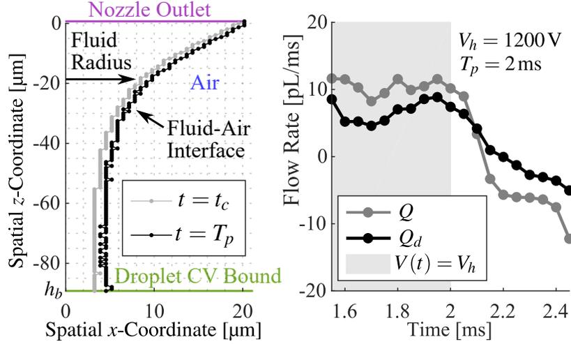
Figure 2.12: Measured data from a particular ejection video illustrating the motivation for a proportional  $Q_d$  model. *Left*: Half-outline of fluid body (the jet is roughly symmetric about  $z$ -axis) at the onset of contiguity and at the end of the voltage pulse, representing a 7% increase in volume outside the droplet CV. *Right*: Flow rate time series data during contiguity illustrating roughly proportional signals between  $Q$  and  $Q_d$ .
