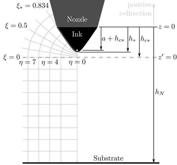
Figure 2.4: To-scale schematic of a critically deformed meniscus and the prolate spheroidal coordinate system (with horizontal axis at  $z' = 0$ ) used to describe the geometry of the meniscus and its local electric field (ellipses) and electric potential contours (hyperbolae). The focus is marked by the white dot at  $z' = a$ . For  $z' < 0$  the field and potential contours are assumed “Cartesian.” Note that by the  $z$ -axis sign convention,  $h$ -values are negative, and  $a$  is positive.
