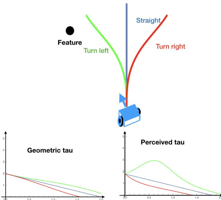
Fig. 2. When time-to-transit,  $\tau$  is computed using pixel motions on the retina, values deviate from the corresponding geometric quantities. Here, the vehicle turns slightly toward the feature as it rises toward the top of the figure along the green path. While the geometry of this motion clearly increases  $\tau$  relative to what it would have been traveling at the same speed along the straight (blue) path, the perceived value increases considerably more.
