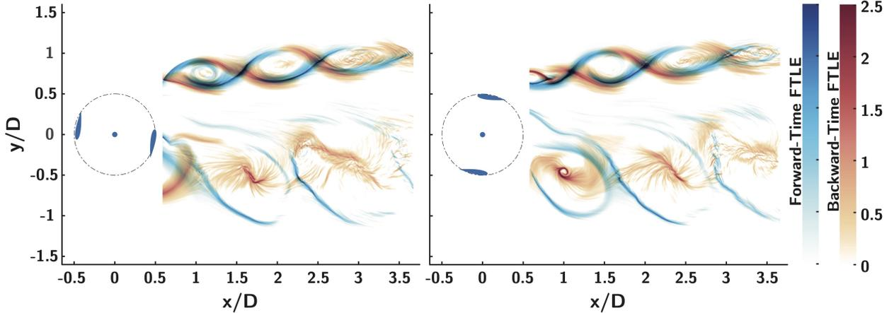
Figure 9: Forward and backward FTLE fields computed on  $\bar{\mathbf{u}} + \tilde{\mathbf{u}}$  (optDMD method). These fields represent areas of maximum stretch and convergence respectively, and together outline the boundaries of coherent structures.
