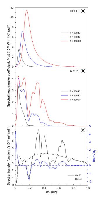
Figure 4. Multiband transport in TBLG. Spectral heat transfer coefficient for (a) DBLG and (b) TBLG with  $\theta = 2^{\circ}$  at room and higher temperatures, with  $\mu = 0$  eV and d = 10 nm. The spectral transfer function (left) for DBLG and TBLG with  $\theta = 2^{\circ}$ , and the imaginary part of the optical conductivity of TBLG (right). The dashed blue line indicates Im  $\sigma = 0$ .
