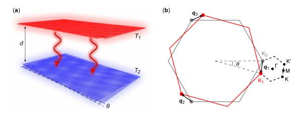
**Figure 1.** (a) Schematic of radiative thermal transport between two identical TBLG sheets separated by a vacuum gap. (b) Reciprocal space of TBLG. The red and gray hexagons represent the first Brillouin zones for the two layers.  $K_1$  and  $K_2$  are the Dirac points. The dashed black hexagon shows the Moiré Brillouin zone with the high symmetry points labeled.  $q_j$  represents the nearest-neighbor interlayer hopping process.
