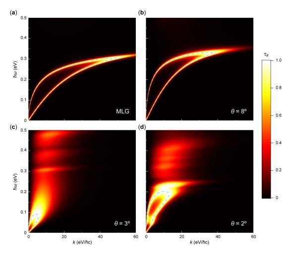
Figure 5. Photon tunneling probability across a 10 nm gap at  $\mu = 0.25$  eV. (a) MLG. (b)-(d) TBLG with  $\theta = 8^{\circ}$ ,  $3^{\circ}$ , and  $2^{\circ}$ , respectively. The dashed cyan lines represent the dispersions of coupled SPPs.
