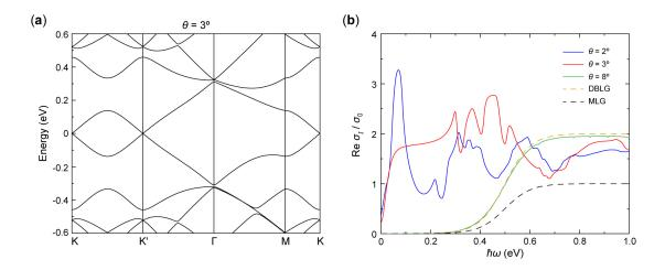
**Figure 2.** (a) The calculated electronic band structure of TBLG with a twist angle of 3°. (b) Real part of the interband optical conductivity of MLG, DBLG, and TBLG with representative twist angles.  $\sigma_0 = e^2/4\hbar$  is the universal conductivity of MLG.
