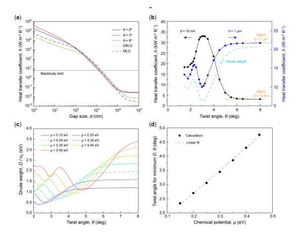
**Figure 3. Twist-angle-dependent NFRHT.** (a) Heat transfer coefficient as a function of gap size for representative cases at T = 300 K and  $\mu = 0.25$  eV. (b) Heat transfer coefficient as a function of twist angle for d = 10 nm and d = 1 µm. The dashed cyan curve shows the corresponding Drude weight. (c) Variation of Drude weight with twist angle at different chemical potentials, and (d) the respective twist angle for minimum Drude weight. The gray dashed line is a linear fit.
