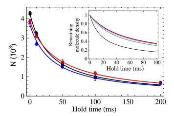
FIG. 2. Loss of <sup>23</sup>Na<sup>87</sup>Rb in the cw ODT (black squares) and chopped ODTs modulated at 1 kHz (red dots) and 2 kHz (blue triangles) with the optical chopper. The duty cycle is  $\eta = 33\%$ . Error bars show the standard error. Inset: Simulated <sup>23</sup>Na<sup>87</sup>Rb loss curves in the cw (bottom black curve) and chopped traps with  $\eta = 33\%$ . From top to bottom  $f_{\rm mod}$  are red: 1 kHz, blue: 2 kHz, orange: 4 kHz, and cyan: 8 kHz for comparison.
