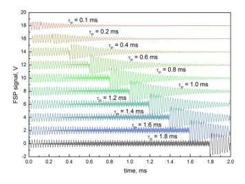
FIG. 5. (Color online) Time dependences of free precession signals at different optical pumping intervals.
