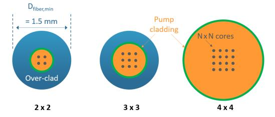
Fig. 3: Schematics of MCFs with different core and cladding configurations. The pump cladding (orange) with a low index layer (green) is adapted in each simulated case to achieve the same small signal pump absorption of 20 dB/m. The outer fiber diameter is at least 1.5 mm, but when the pump cladding (orange) is larger than this value, the outer fiber diameter has the same dimension as the pump cladding.
