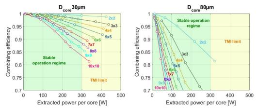
Fig. 7: Combining efficiency vs. extracted power per core for different MCFs with (left) 30µm and (right) 80µm core diameter. The green and yellow shaded areas represent the regime of stable operation and TMI, respectively.
