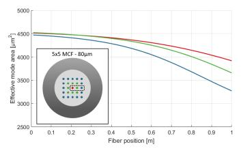
Fig. 4: Evolution of the effective mode area of the propagating fundamental modes in three different cores (indicated by the dashed rectangle in the inset) along a 5x5 MCF with 80  $\mu$ m cores, counter pumped with an average output power of 3.4 kW. The inner core (red line – also colored red in the inset) shows less shrinking than the middle core (green) and the outer core (blue).
