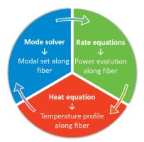
Fig. 2: Schematic flow-diagram of the simulation tool.
