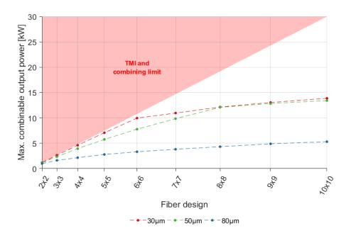
Fig. 8: Maximum combinable output power for the different MCFs (2x2 to 10x10) with different core sizes (30, 50 and 80  $\mu$ m). The red shaded area represents operation beyond the TMI threshold of 300 W per core together with a 100% combining efficiency.
