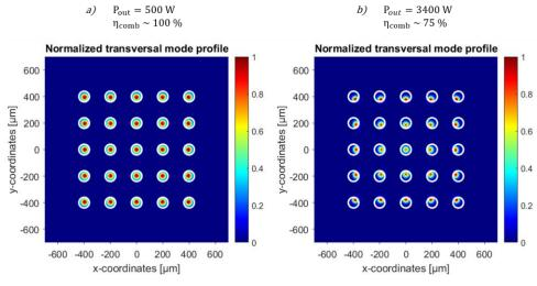
Fig. 5: Example of intensity profiles in a 5x5 MCF (80 μm cores) at different power levels. In a) ~100% of combining efficiency is achieved whereas in b) due to non-uniform mode shrinking just ~75% of combining efficiency is obtained.
