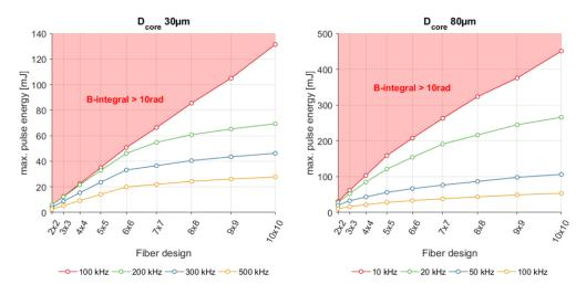
Fig. 9: Maximum achievable pulse energy at different repetition rates for 30µm (left) and 80µm (right) MCFs.
