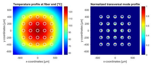
Fig. 1: Exemplary temperature profile (left) and corresponding transversal intensity profile (right) in a 5x5 active MCF under heat load, with cores highlighted as white circles.
