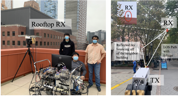
Fig. 6: The RX is at heights of 1.5 m above the roof corner, which prevents the RX from being shadowed by the railing boundary, emulating a passive receiver in a satellite. The TXs are at heights of 1.5 m above ground working as mobile terminals.
