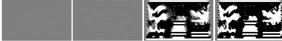
Figure 14: Differences between truth and reconstructed images of the bar phantom with DTV (columns 1 & 2) and ITV (columns 3 & 4) algorithms from data over an angular range of 20^\circ . Display window: [-10^{-2}, 10^{-2}] \text{ cm}^{-1} for columns 1 & 3, [-10^{-3}, 10^{-3}] \text{ cm}^{-1} for columns 2 & 4.
