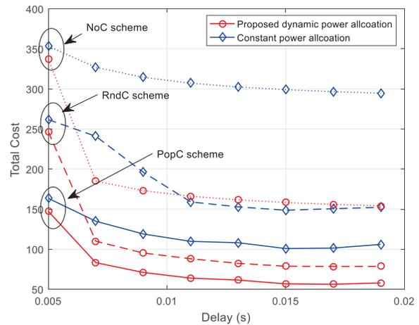
Fig. 4. Total power cost for different delay requirements at an average SNR  $\frac{P_{1,avg}}{\sigma^2} = \frac{P_{2,avg}}{\sigma^2} = 10$  dB.
