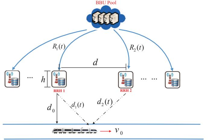
Fig. 1. Fog-RAN-assisted high-speed communication system.
