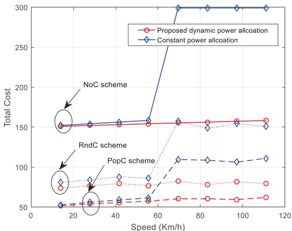
Fig. 6. Total power cost for different train speeds at an average SNR  $\frac{P_{1,\text{avg}}}{\sigma^2} = \frac{P_{2,\text{avg}}}{\sigma^2} = 10$  dB.
