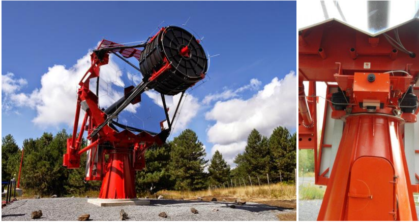
Fig. 1 ASTRI-Horn, the dual-mirror Cherenkov telescope installed on Mt.Etna, Italy, at the INAF 'M.C. Fracastoro' observing station. On the right panel it is visible the small UVscope instrument mounted under the primary mirror structure of the ASTRI-Horn telescope.
