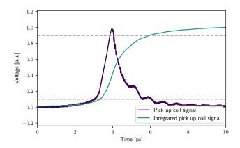
FIG. 4. Fast change of the magnetic field of the fast coil. The pick-up signal (purple) and its integrated signal (blue) during the magnetic field switching, the dashed lines indicate 10% and 90% voltage levels of the integrated signal. The time of the magetic field change is about  $3\,\mu s$ .
