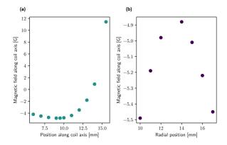
FIG. 2. Profile of the magnetic field of the fast coil. (a) Magnetic field along z direction. (b) Magnetic field in radial directions of the coil at  $z_0 = 9$  mm. All the fields are measured at a current of 5A through the coil. The magnetic field at 40A is verified to be 36 G by Zeeman spectroscopy with atoms.
