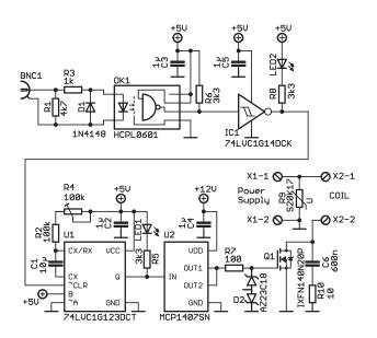
FIG. 3. Schematic of the control circuit of the fast coil.
