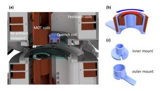
FIG. 1. Experimental setup and coils. (a) Schematic drawing of the metallic vacuum chamber and magnetic field coils. The red dot indicates the atoms in the chamber. (b) Design of the fast coil. The blue and red arrows show the current through the coils. (c) CAD drawing of the 3D printed mount of the coils.
