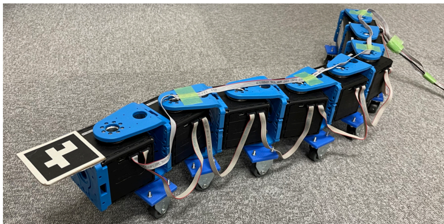
Figure 7 Snake robot with eight VSAs serially connected: as its actuator, we use Qbmove developed QbRobotics, which can control its stiffness; this robot is on casters to easily drive forward by snaking locomotion, base of which is generated by CPGs.
