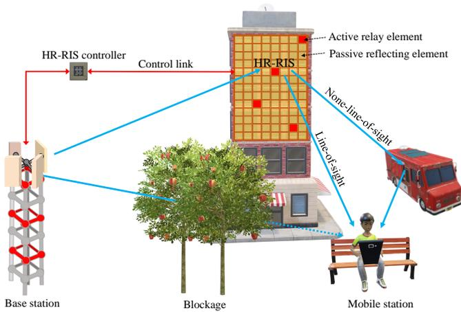
Figure 1: Illustration of an HR-RIS-aided wireless communication system.
