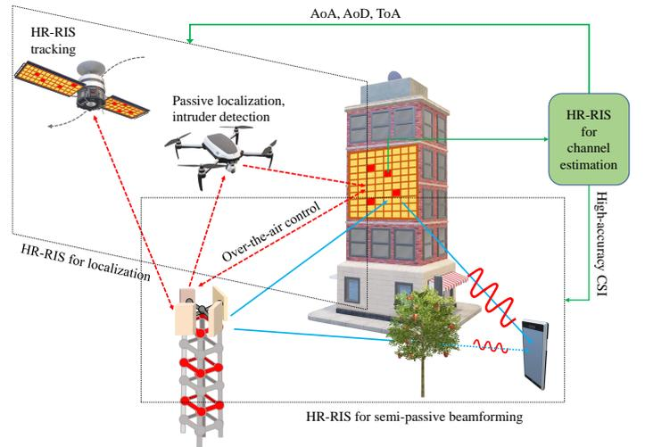
Figure 3: Application of HR-RIS to semi-passive beamforming, channel estimation, and localization.
