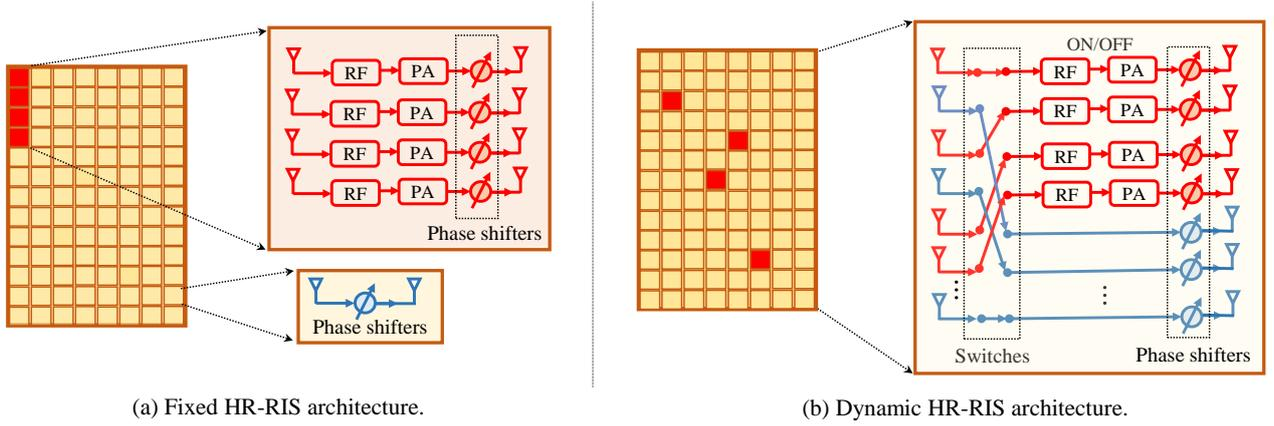
Figure 2: Illustration of (a) fixed and (b) dynamic HR-RIS architectures.
