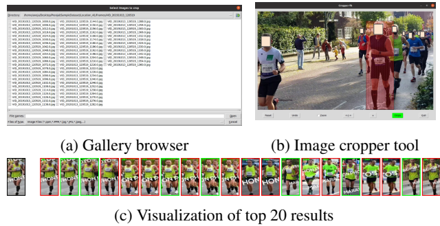
Figure 26: An outlook of the person re-identification tool integrated with runners' dashboard. (a) The tool offers the option to quickly browse images from the gallery set. (b) The target runner can be cropped from the selected image. After cropping, the person re-id system will be activated for the cropped person's image. (c) The top-20 matches closest to the probe images are displayed as the final output.
