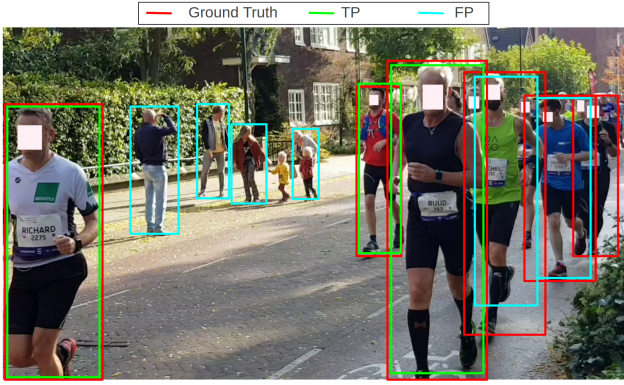
Figure 14: An example of True positive (TP), False positive (FP), and False negative (FN) case. The boxes in red color represents the ground truth. whereas boxes in green are TPs and in blue are FPs. Runners that didn't get detect are FNs, represented by only red box.
