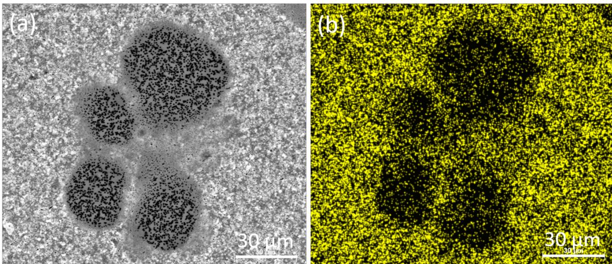
**Figure 6. Resorption pits on ammonia-induced calcium phosphate coating surface.** (a) BSE image of resorption pits (dark area) and calcium phosphate coating (bright area). (b) EDS mapping of calcium.
