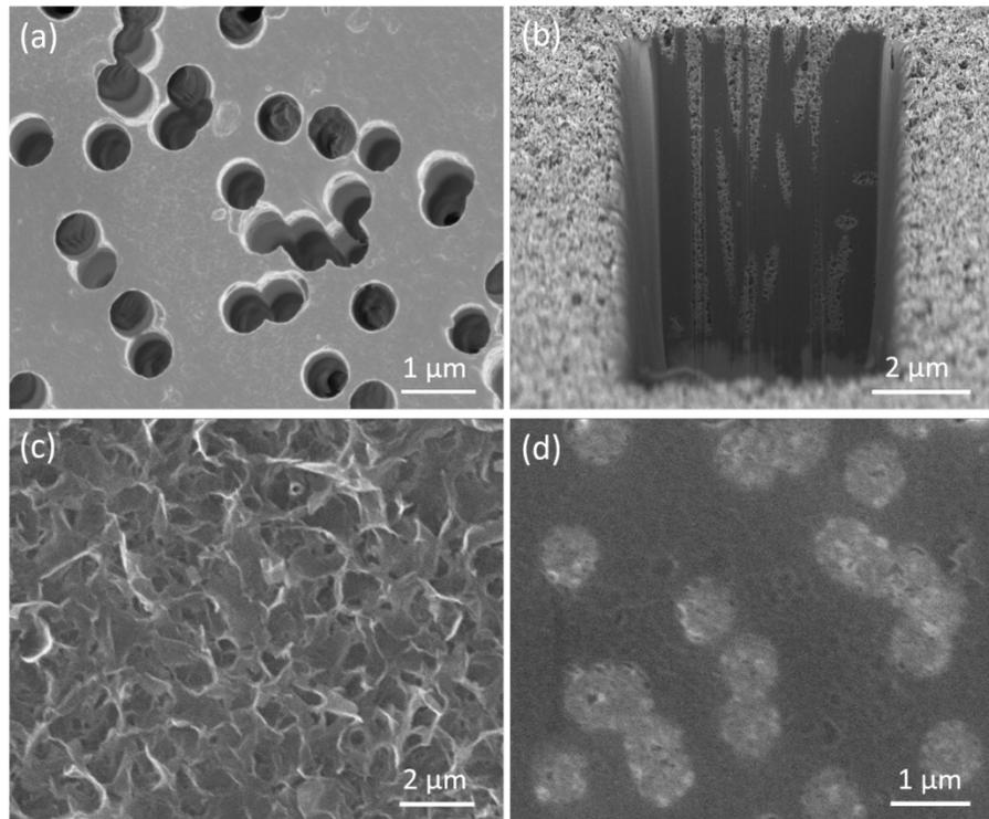
**Figure 2.** SEM images of the original track-etched Falcon® cell culture insert membrane showing nanopores of 400nm in diameter (a); focused ion beam cross section showing calcium phosphate minerals forming coating on membrane surface and filling the throughout pores (b); (c) calcium phosphate coating on the inner surface of insert; (d) outer surface of the insert showing calcium phosphate (bright phase) only filling the pores.
