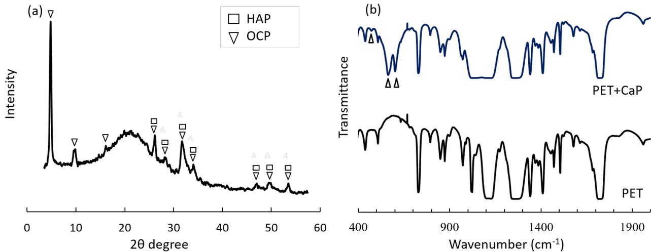
**Figure 3. Chemical composition of ammonia-induced CaP coating.** (a) XRD spectrum of the calcium phosphate coating on the inner surface of insert; (b) FTIR spectra of the calcium phosphate coating on insert membrane surface (PET+CaP) and original insert membrane (PET). Triangles mark CaP peaks.
