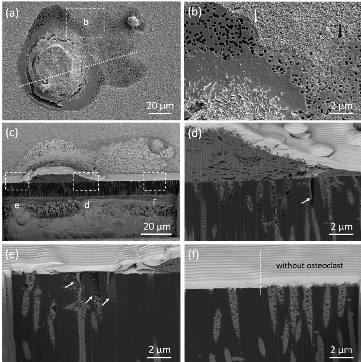
**Figure 5. SEM and FIB images of osteoclast interaction on calcium phosphate coating.** (a) Top view of osteoclast and its resorption pit on ammonia-induced calcium phosphate coating. Focused ion beam cut the cells and membrane along the white dot line. (b) Magnified resorption areas of osteoclast. The white arrow indicated deep resorption pit, and the black arrow indicated the shallow resorption pit. (c)
