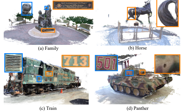
Figure 8: Visualization of the generated 3D point clouds without any finetuning on Tanks&Temples dataset.
