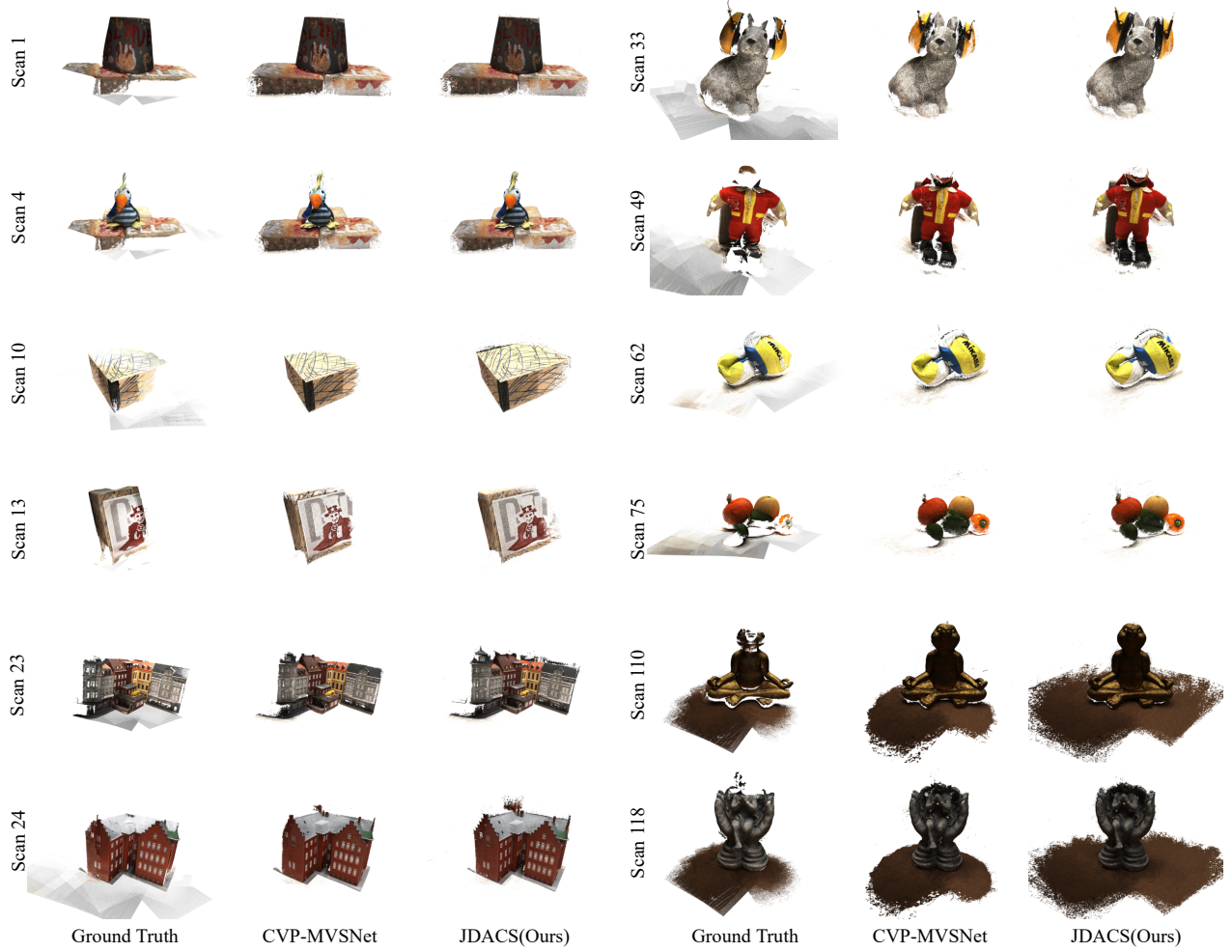
Figure 10: More qualitative comparison in 3D reconstruction between our JDACS and SOTA supervised method (CVP-MVSNet) on DTU dataset. From left to right: ground truth, results of CVP-MVSNet, our results.
