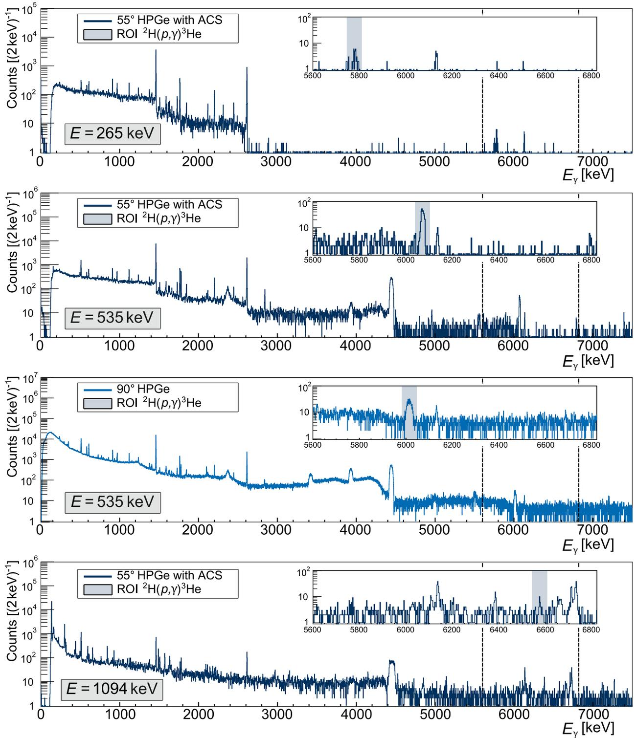
FIG. 6.  $\gamma$ -ray spectra at the lowest and highest energies studied,  $E = 265$  and  $1094$  keV, respectively, and at a representative intermediate energy  $E = 535$  keV. The shaded areas inside the insets show the beam energy and detector angle dependent region of interest for the  ${}^2\text{H}(p,\gamma){}^3\text{He}$  peak. See text for details.
