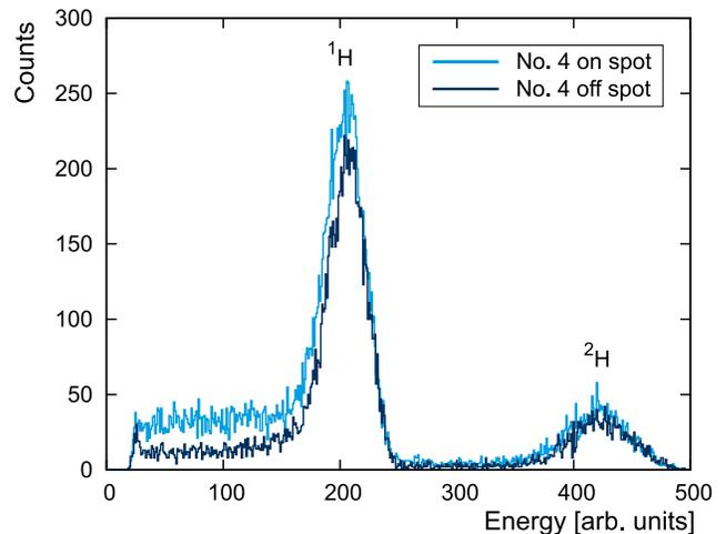
FIG. 4. Pulse height spectra of the silicon detector used for determining the  $^1,^2\text{H}$  content in the ERD runs, for target No. 4, inside and outside the respective proton beam spot. The two runs have similar incident charge but the spectra were not normalized.
