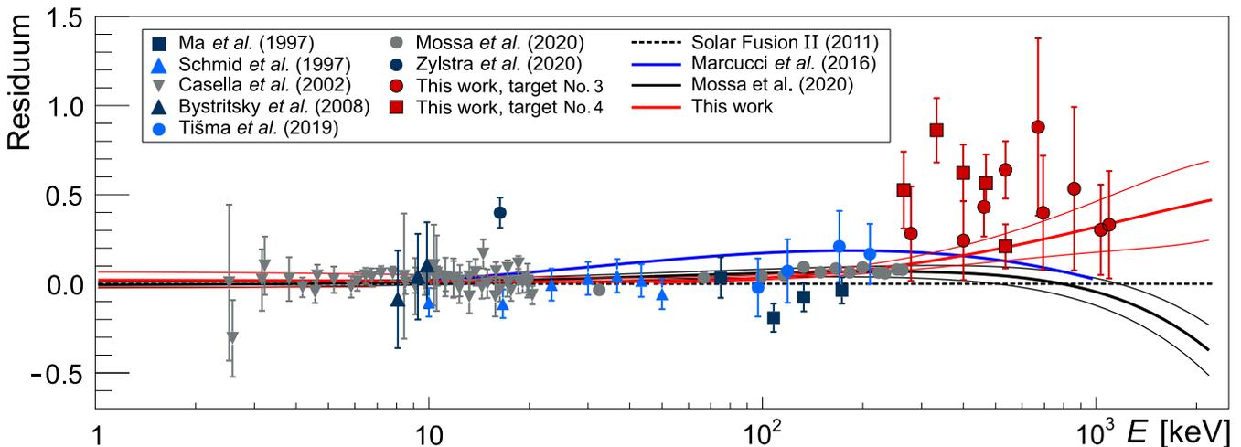
FIG. 9. Residuum of the S-factor data [13–19, and present work] with respect to the Solar Fusion II fit [21]. The *ab initio* theory curve by Marcucci [22], the Mossa *et al.* fit [17], and the present fit are also shown (blue, black, and red, respectively). The standard deviation ( $1\sigma$ ) of the present fit is given by thin red lines. The error bars for the data points are only statistical.
