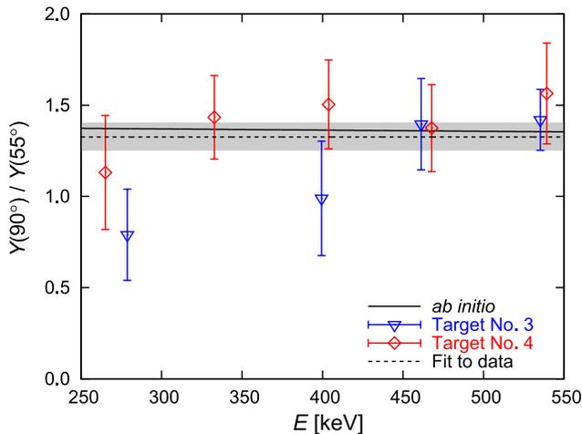
FIG. 7. Ratio of the efficiency-corrected yields  $Y^*$  of both HPGe detectors as a function of center-of-mass energy  $E$ . The *ab initio* predicted yield ratio is shown as a solid line [22, 43, 44]. The dashed curve and shaded area are a constant fit to the data and its uncertainty. See text for details.
