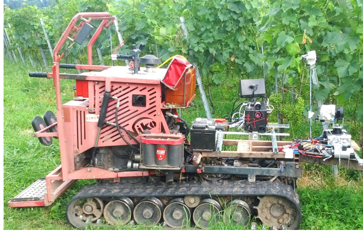
Figure 2: Niko caterpillar vehicle used for experimentation equipped with a multi-sensor suite.
