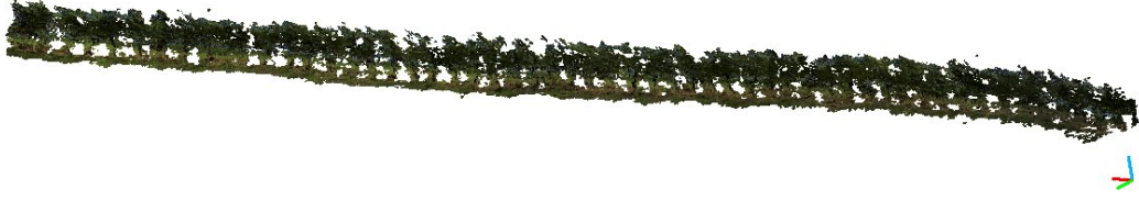
Figure 9: 3D reconstruction of the grapevine row under inspection. It includes 55 plants spanning along a total length of approximately 50 m. Plants are located at approximately 0.90 m apart with respect to each other.
