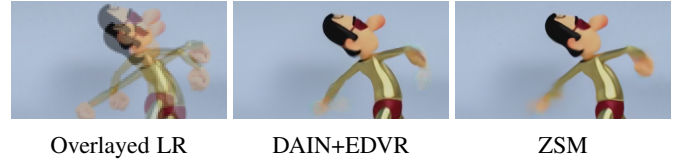
Fig. 14: Failure example. Our model might fail to handle dynamic video objects with severe geometric deformations.
