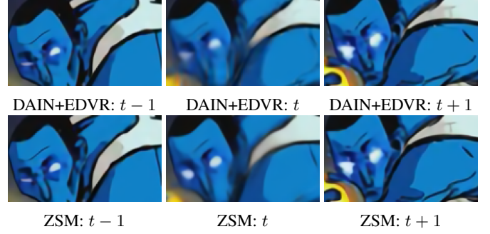
Fig. 13: Temporal inconsistent issue in STVSR. It is more difficult to synthesis HR frame t than HR frames: t-1 and t+1 , since LR frames: t-1 and t+1 are available and LR frame t is missing during testing. Synthesized HR frame at the time step t is more blurry with fewer visual details than results at t-1 and t+1 .
