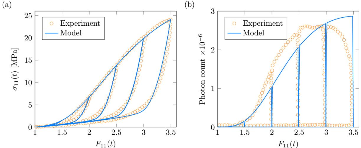
Figure 6: (a) Mechanical response of the triple ethyl acrylate network (EA<sub>0.5</sub>EAEA) of Ducrot et al. (2014) under cyclic uniaxial tension, and that predicted by the rate-independent irreversibly-breaking model. (b) Light emission from the sacrificial mechanoluminescent crosslinkers breaking within the first network in the same experiment, and that predicted by the model.
