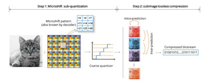
Fig. 1. Compression overview. The first step quantizes the micro-shifted image with M bits. The second step compresses the subimages sequentially.
