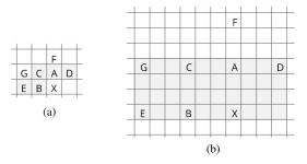
Fig. 6. Prediction template. (a)  $A \sim E$  in the subimage  $\tilde{I}^{(1)}$  are used for intra-prediction. (b) the locations of template pixels in the original image  $\tilde{I}$ . Rows that are buffered for are denoted in shaded gray.
