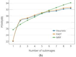
Fig. 8. Progressive decompression. *Microshift* uses the parameters N = 3, M = 3 for compression. (a) With longer bitstream of subimages received, the decompressed quality gradually increases. (b) The PSNR increases as more subimages are used for decompression.
