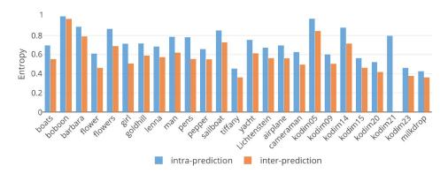
Fig. 9. Entropy for intra-prediction and inter-prediction when encoding the subsequent subimages. Lower entropy indicates better compression performance.
