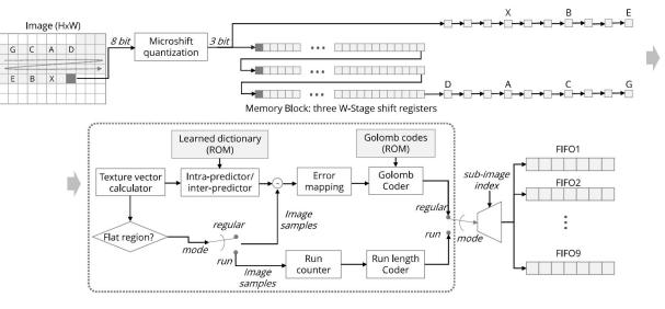
Fig. 10. The diagram of hardware implementation.
