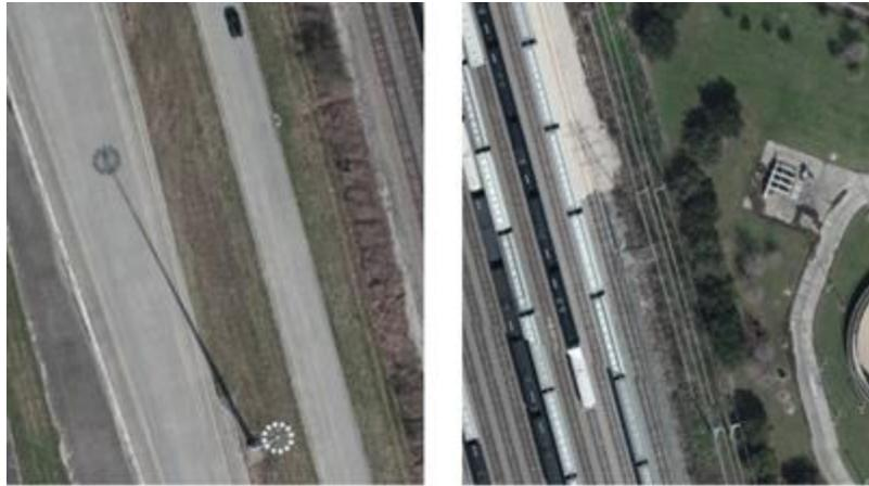
**Figure 13.** Sample failed cases where the model misses the presence of an object completely. The cases are magnified regions from the second RGB image (second row) of Figure 10. The image on the left shows a very high pole standing on a highway with a height of 30 meters (according to its Lidar measurement). Despite the pole's long shadow, the model does not detect it. The magnified region on the right contains a tall electric energy transmission tower that goes undetected by the model.
