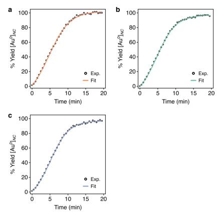
**Figure S7.** Kinetics of NC growth analyzed via the peak nanoplasmonic absorbance. Colloidal Au nanocubes were grown with (a) 0.1 equivalents (eqv.) NaOH, (b) 1 eqv. HCl or (c) 2 eqv. HCl. The data were fitted to Eq. (11) ( $r^2 > 0.99$  for each).
