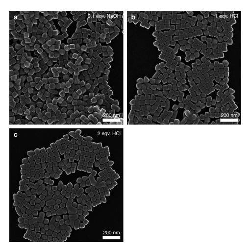
**Figure S6.** Large-area SE-STEM images of Au nanocubes after growth. The micrographs show the NCs grown with (a) 0.1 equivalents (eqv.) NaOH, (b) 1 eqv. HCl or (c) 2 eqv. HCl.
