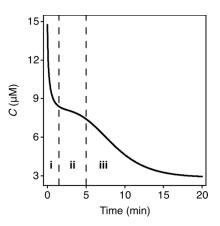
**Figure S2.** Estimated concentrations of monomer throughout growth. This profile was estimated using eq. (1) and the profile of the supersaturation dynamics shown in Figure 3e.
