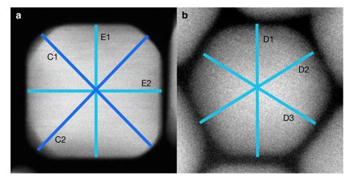
**Figure S3.** Schematic representations of NC sizing measurements from STEM images. (a) Cubes were characterized by corner-to-corner (C) and edge-to-edge (E) distances. (b) Cuboctahedra were characterized by side-to-side (D) distances.
