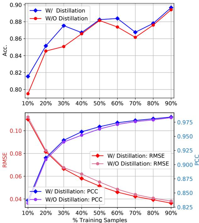
Fig. 3: The performance of the student network with different number of training samples for SEED (**top**) and SEED-VIG (**bottom**) datasets, respectively. Comparison is performed for networks trained with distillation (labeled as 'W/ Distillation') and networks trained from scratch without distillation (labeled as 'W/O Distillation').
