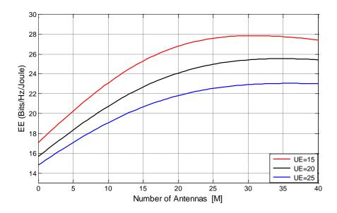
Figure 3. Energy efficiency versus transmit a number of antennas in small cells.
