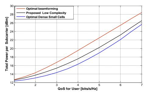
Figure 2. Related transmit power with a quality of service in dense small cells.
