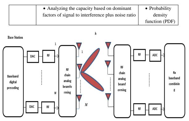
Figure1. Hybrid analogue-digital architectures in a massive MIMO channel.
