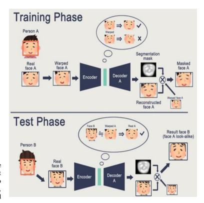
Fig. 4. Working procedures of autoencoder.
